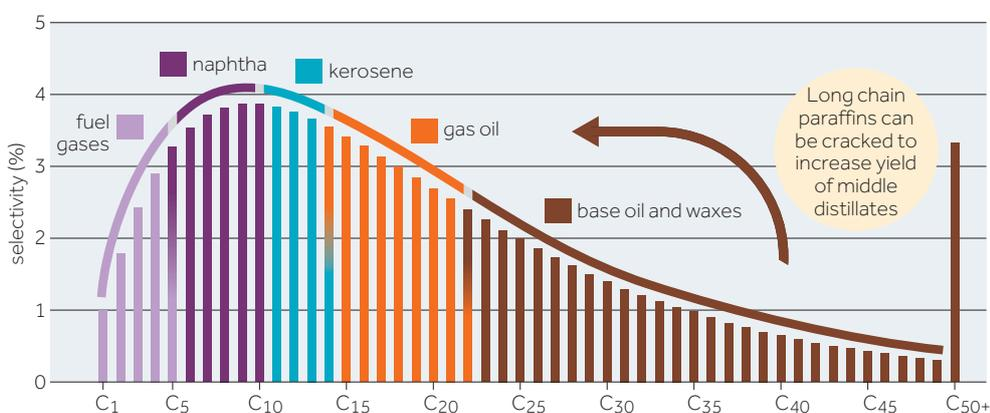
The resulting 'e-crude' from the Fischer-Tropsch reaction, which can be a single stream or several separate streams, could be fed to a hydrocracking unit. The intermediate wax molecules are hydro-processed within a hydrocracker into shorter 'middle distillate' molecules, which are then purified by distillation into naphtha, kerosene and gas oil fractions.
