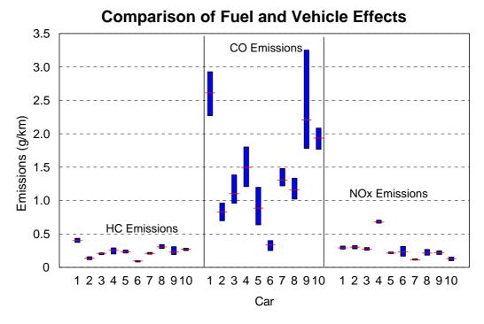
The variation across the fuels for each car is represented by the vertical bars. The horizontal line indicates the mean emissions for each car averaged over the seven fuels. The ten cars are represented for each emissions species across the horizontal axis
