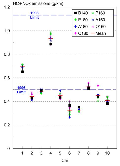
The asterisks and crosses show the emissions for each of the seven fuels in each car. The red + shows the mean emissions for each car over the seven fuels.
