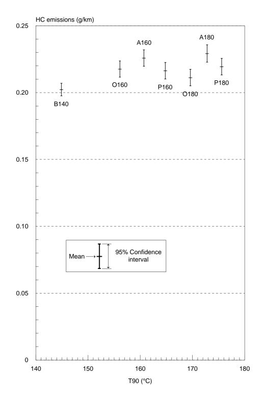
*Figure 7* Total cycle HC Emissions (Ten-car Geometric Mean)
