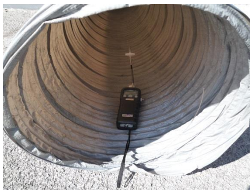
Figure 7: Positioning of PID analyzer in the wind tunnel exhaust.
