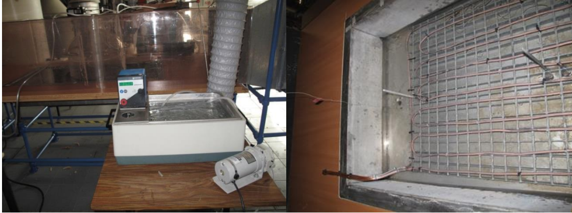
Figure 5: Water heating system.
