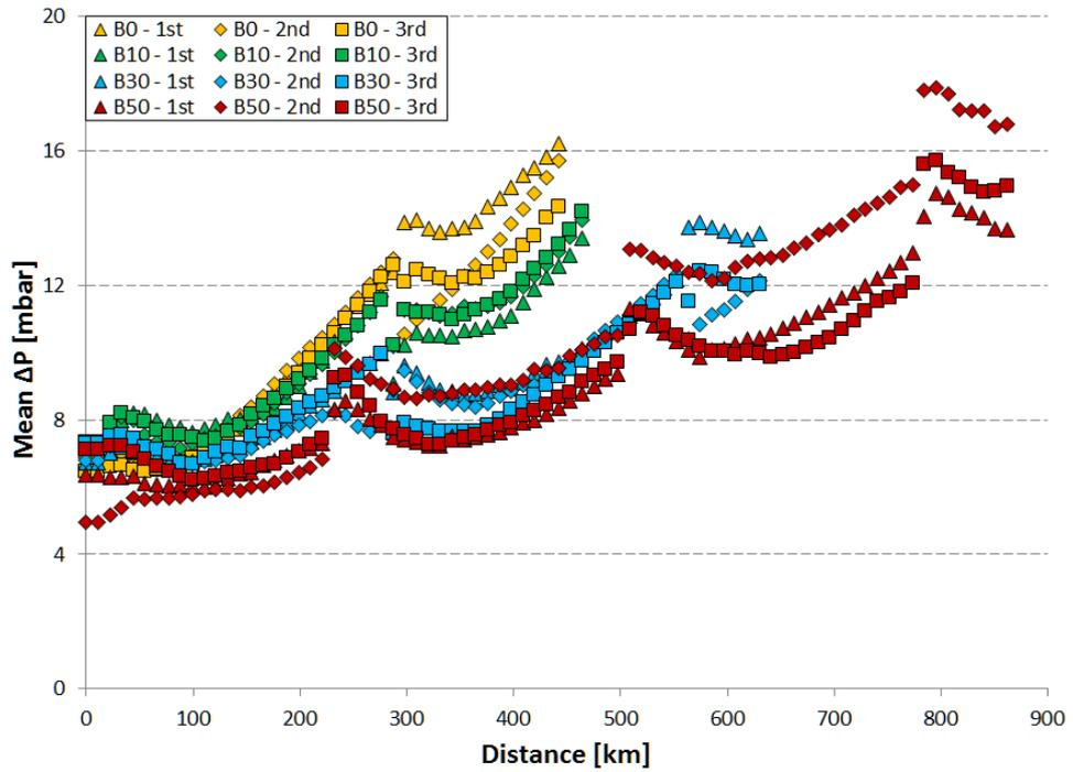
**Figure 5.** Maximum NEDC pressure drop across the DPF for each fuel blend
