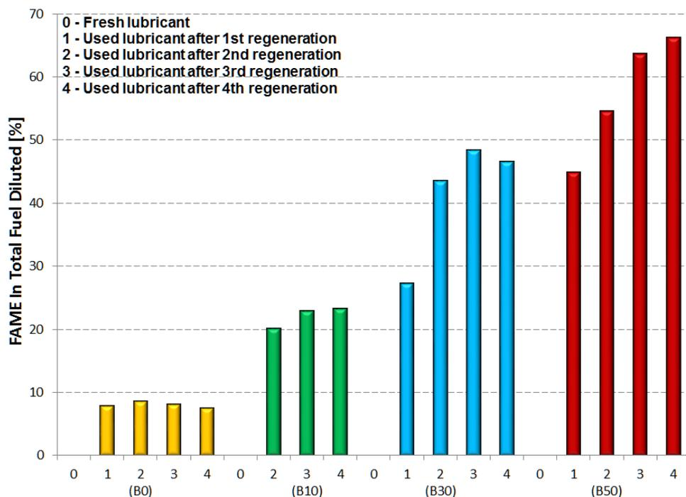
**Figure 11.** Total fuel content (DIN 51454) in the lubricant samples
