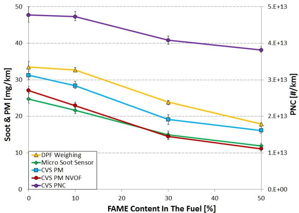
Consistent with the results of Czerwinski et al. [6], the volatile part of the PM emissions increased as the FAME content increased (**Figure 7**).
