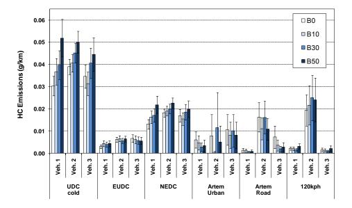
As shown in these figures, the absolute emissions levels for both HC and CO were very low for all vehicles and considerably lower than the Euro 4 regulatory limits. For all hot start cycles, the absolute values for HC were very close to background levels and no statistically significant differences were seen between fuels.
