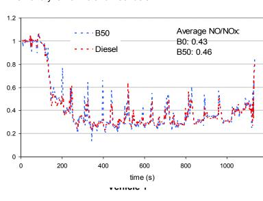
Average instantaneous NO/NOx ratio over NEDC as recorded using the fast NOx analyzer for B0 and B50 fuels
