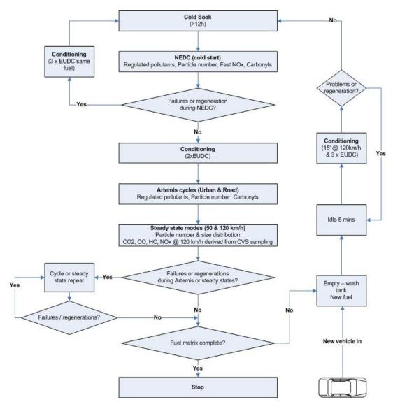
*Figure A4-2* Flowchart of the vehicle test protocol
