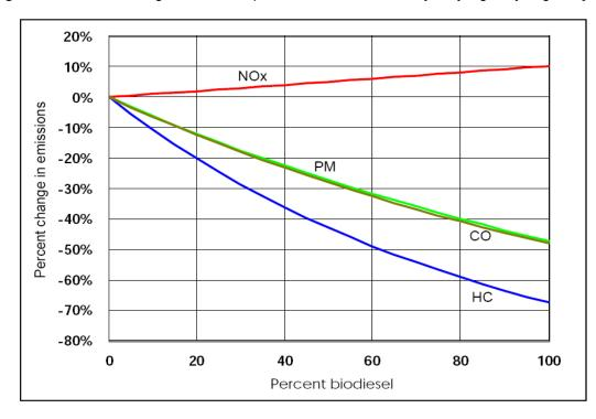
*Figure A2-1* Average emission impacts of biodiesel for heavy-duty highway engines [A2-1]
