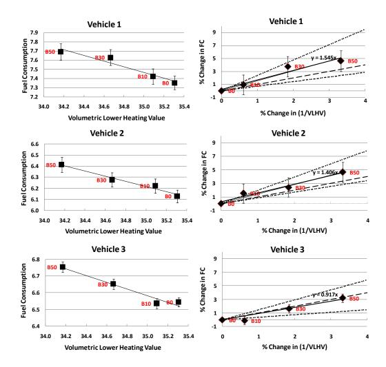
The best fit lines lie above the one-to-one correlation lines for Vehicles 1 and 2, suggesting that the engine efficiency over the NEDC is actually lower on the higher RME fuels. However, these correlation lines are not outside the 95% confidence limits. This means that the change in FC can be simply explained by the loss in energy content of the RME-containing fuels, within the experimental uncertainty inherent in the measurements.
