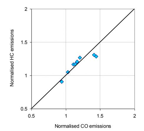
*Figure 21* Normalized HC vs. normalized CO emissions over the UDC cold start cycle
