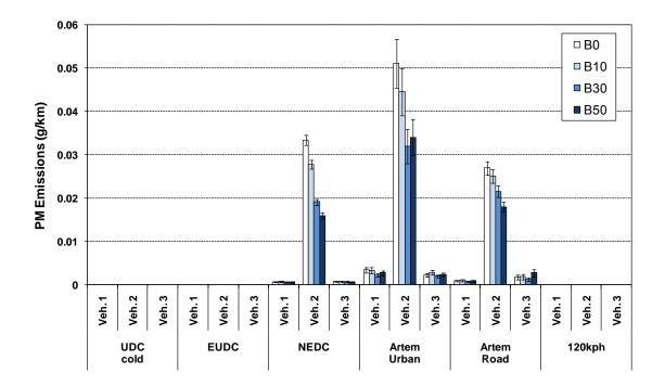
A single filter was used to collect the PM over each complete cycle, including the NEDC. From **Figure 13**, it can be seen that the absolute PM emissions from the DPF-equipped Vehicles 1 and 3 were very low and in some cases close to the measured background. No statistically significant differences were observed from these vehicles with changes in the RME content.
