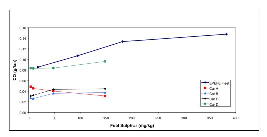
Figure 24 EPEFE Data - Light duty gasoline tests - CO (EUDC)
