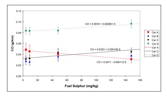
In all cases, emissions during the EUDC part of the cycle were very low. Visual inspection shows that all the sulphur effects are small relative to the prevailing emissions limits. For NOx, there was no statistically significant sulphur effect. For HC, the sulphur effect was significant in Cars A (P<0.1%) and B (P<1%). These effects appear large on a percentage basis but were small on an absolute scale and
