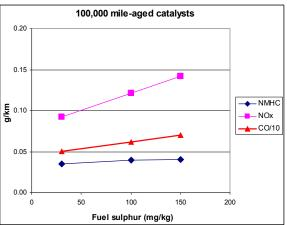
With the catalysts aged to 100,000 miles, all emissions increased compared with the lower mileage catalysts. However, the sensitivity to sulphur, measured here as the percentage emission change between 30 and 150ppm S, stayed the same for HC, increased slightly for CO, but doubled for NOx. It seems, therefore, that NOx emissions are the most sensitive to catalyst condition and ageing.
