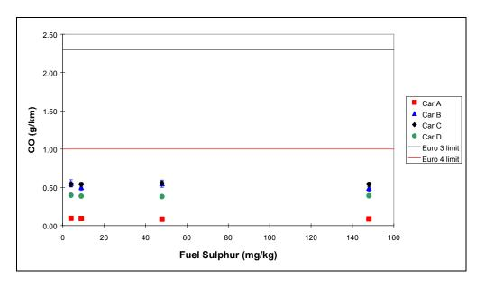
In all four vehicles, there was little short-term response of emissions to fuel sulphur content. There were no statistically significant sulphur effects (P < 5%) over the NEDC cycle for any pollutant in any vehicle, or indeed across the fleet. Furthermore, there is no evidence of higher sensitivity at low sulphur levels.
