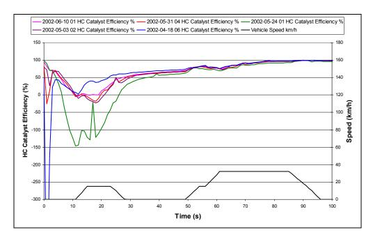
No obvious explanation for this effect could be found, other than that the 3-way catalyst may have adsorbed unburned HC's during the test preconditioning. However, this also seems unlikely given the amount of transient operation and high speed cruising carried out during the preconditioning cycle.
