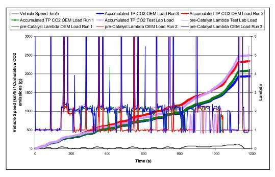
Figure 11 Effect of engine loading on AFR control
