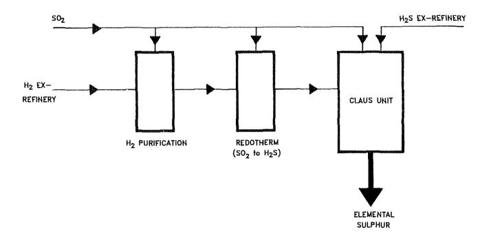
Fig. 4 WELLMAN-LORD PROCESS MASS DIAGRAM
