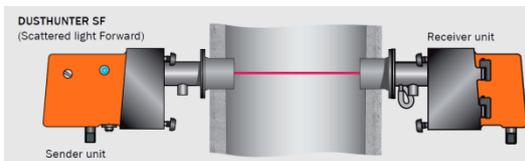
Forward scattering wall mounted devices (SICK, Dusthunter SF)
