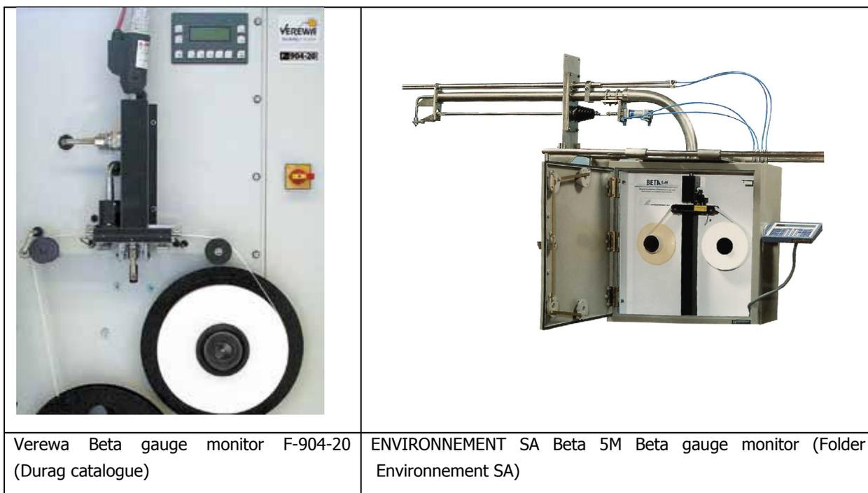
**Figure 9 : Picture of two Beta gauge monitors.**
