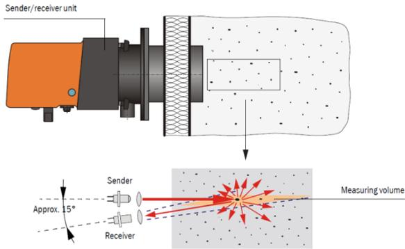
Back scattering wall mounted device (SICK Dusthunter SB)
