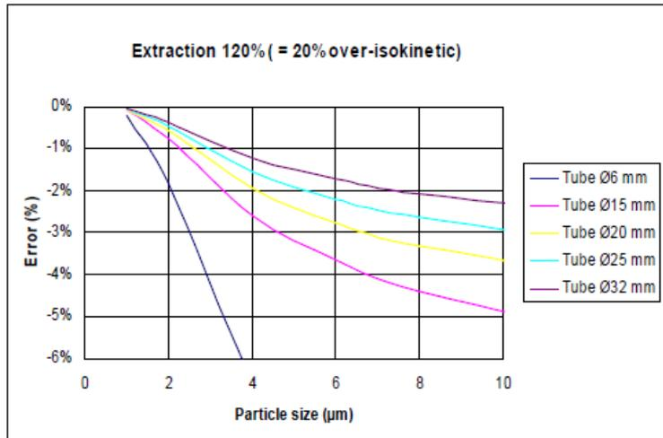
a. Illustration of over-isokinetic sampling and its effects on final result
