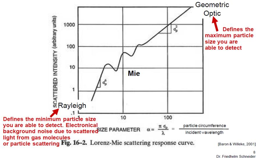
**Figure 6 Physical background- scattering intensity vs. particle size/wavelength (Grimm presentation).**
