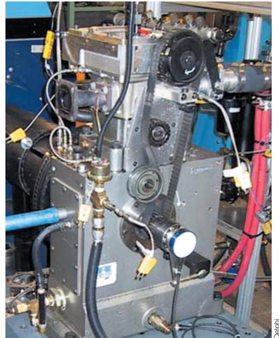
*An early single-cylinder gasoline compression ignition (GCI) test engine developed by Delphi; ongoing development of the GCI concept aims to achieve diesel-like efficiency with low  $\text{CO}_2$  emissions under real-world operating conditions.*
