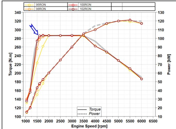
Figure 3. Chart of power and torque output for all fuels.
