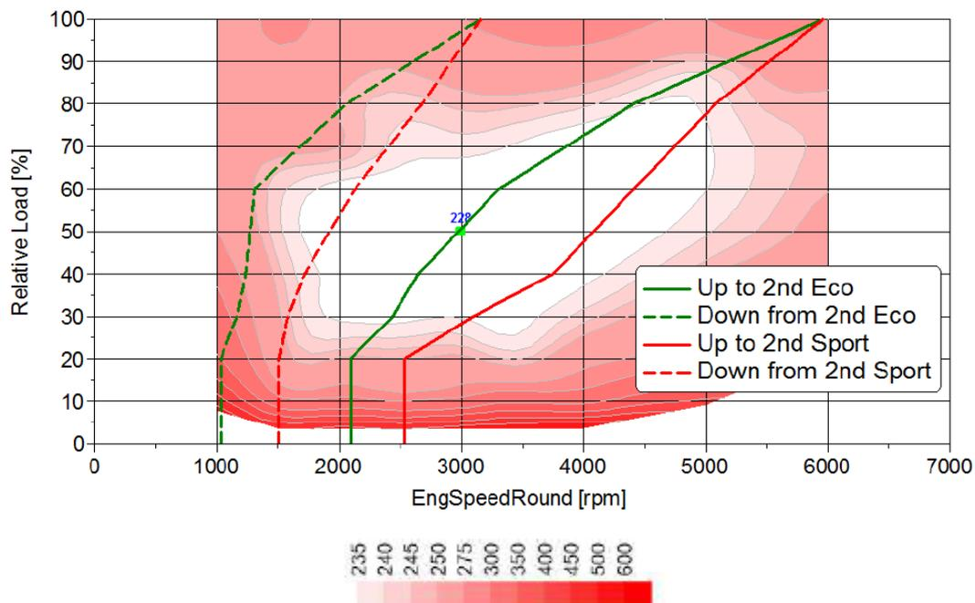
**Figure 15.** Speed-load diagram superimposed on the 102 RON BSFC chart
