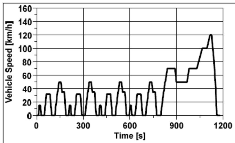
*Figure 6.* The NEDC test cycle
