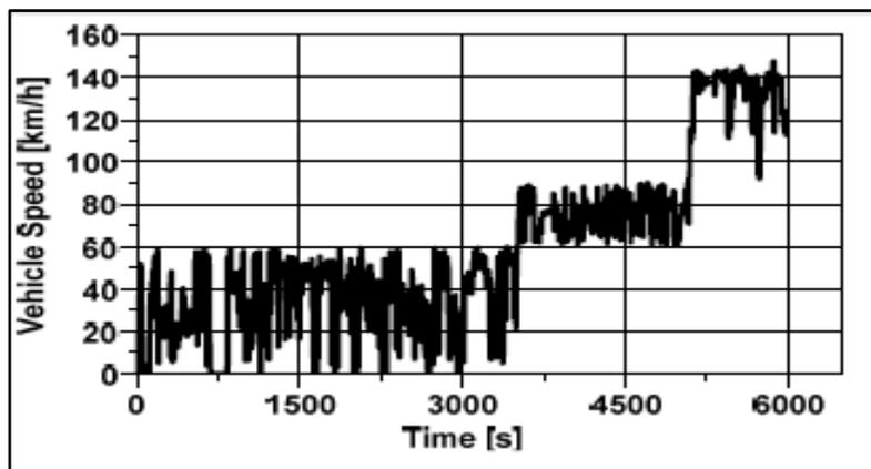
Figure 8. Speed time graph for RDE cycle used
