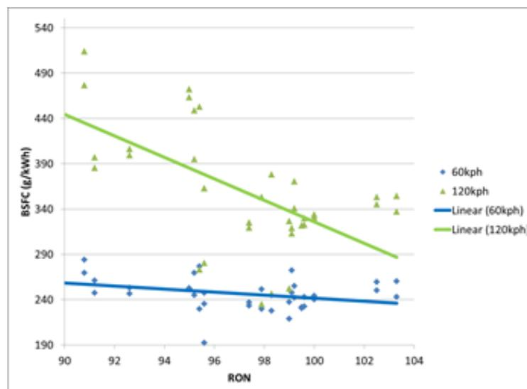
**Figure 1.** Brake Specific Fuel Consumption (BSFC) versus RON for two steady state conditions
