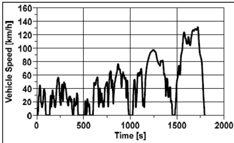
Figure 7. Speed time chart for WLTC
