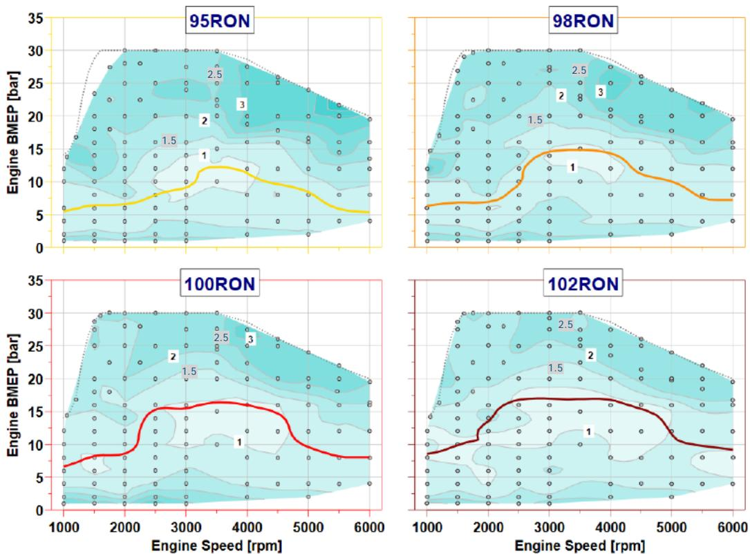
Figure 13. Contour plots for NMEP covariance with knock limit superimposed
