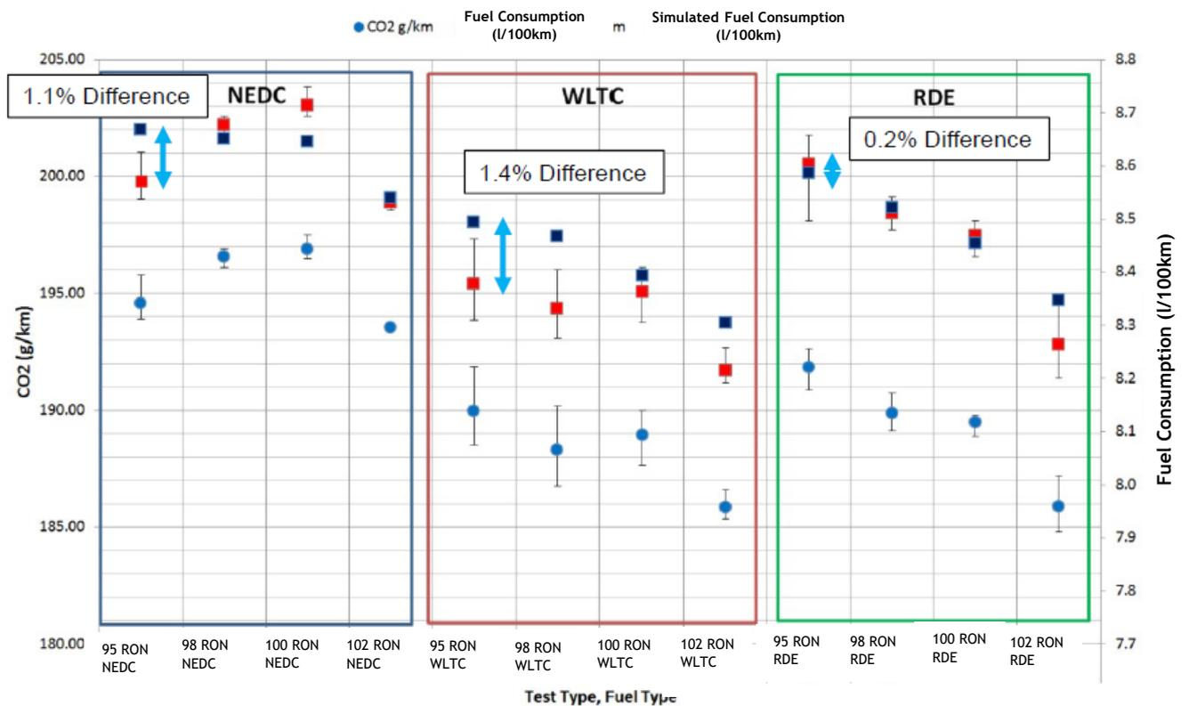
Figure 17. CO<sub>2</sub> and fuel consumption results including modelled fuel consumption results
