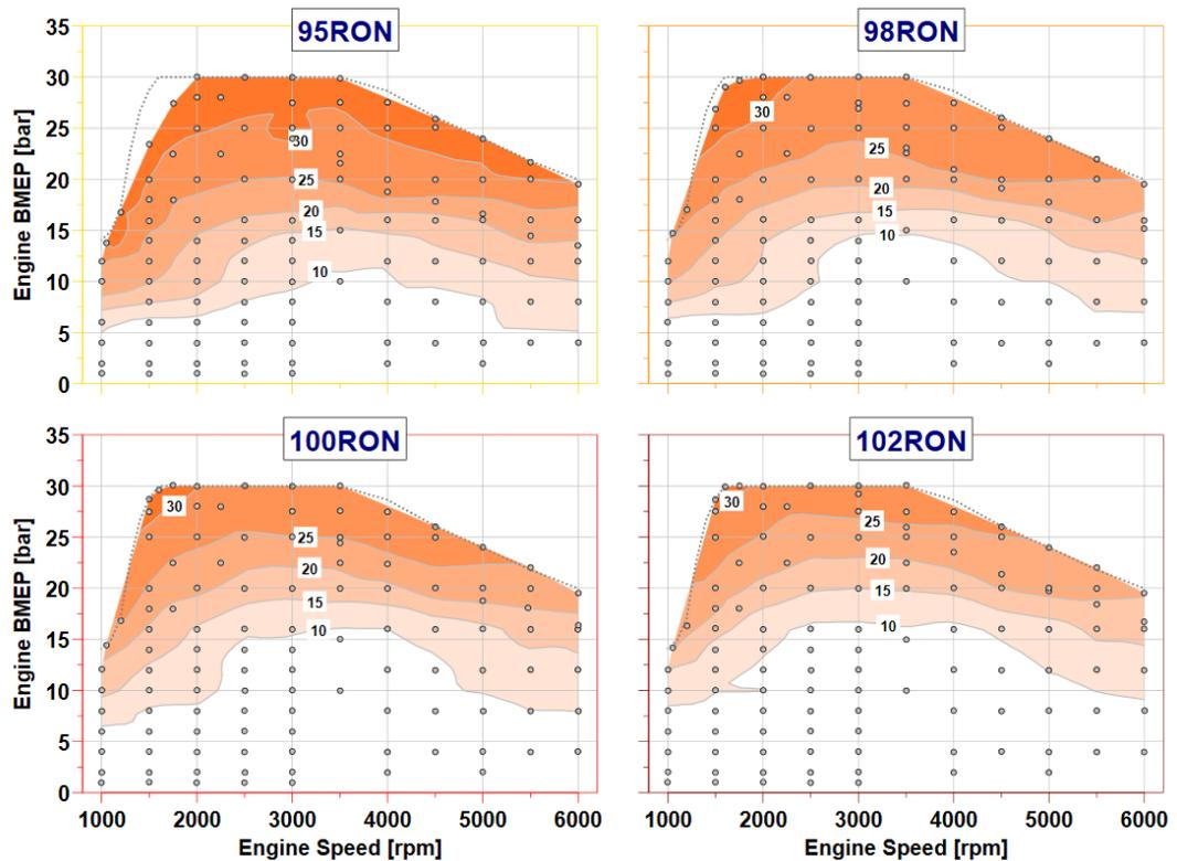
**Figure 5.** Speed vs Load maps of combustion phasing (CA50) for each fuel
