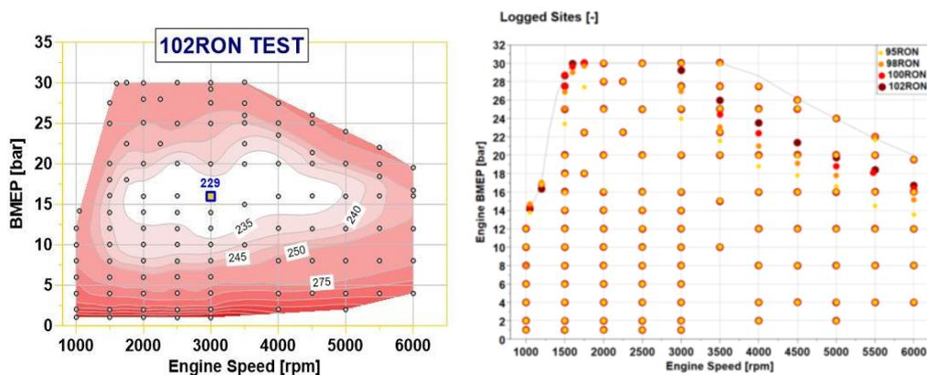
**Figure 4.** Speed vs Load map of a) calibration and b) logging points for all fuels.
