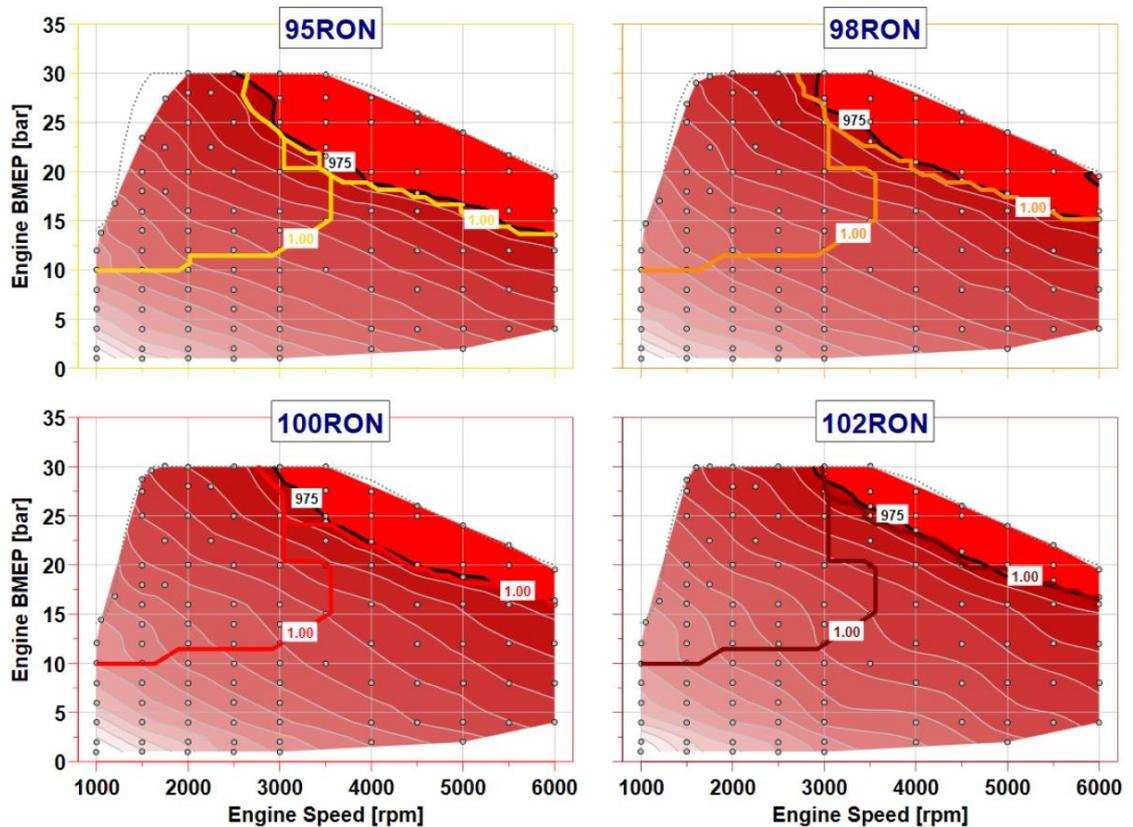
**Figure 11.** Contour plots for exhaust gas temperature
