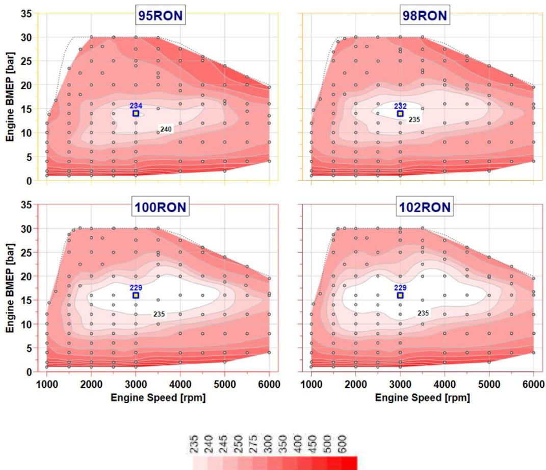
**Figure 10.** Contour plots for brake specific fuel consumption
