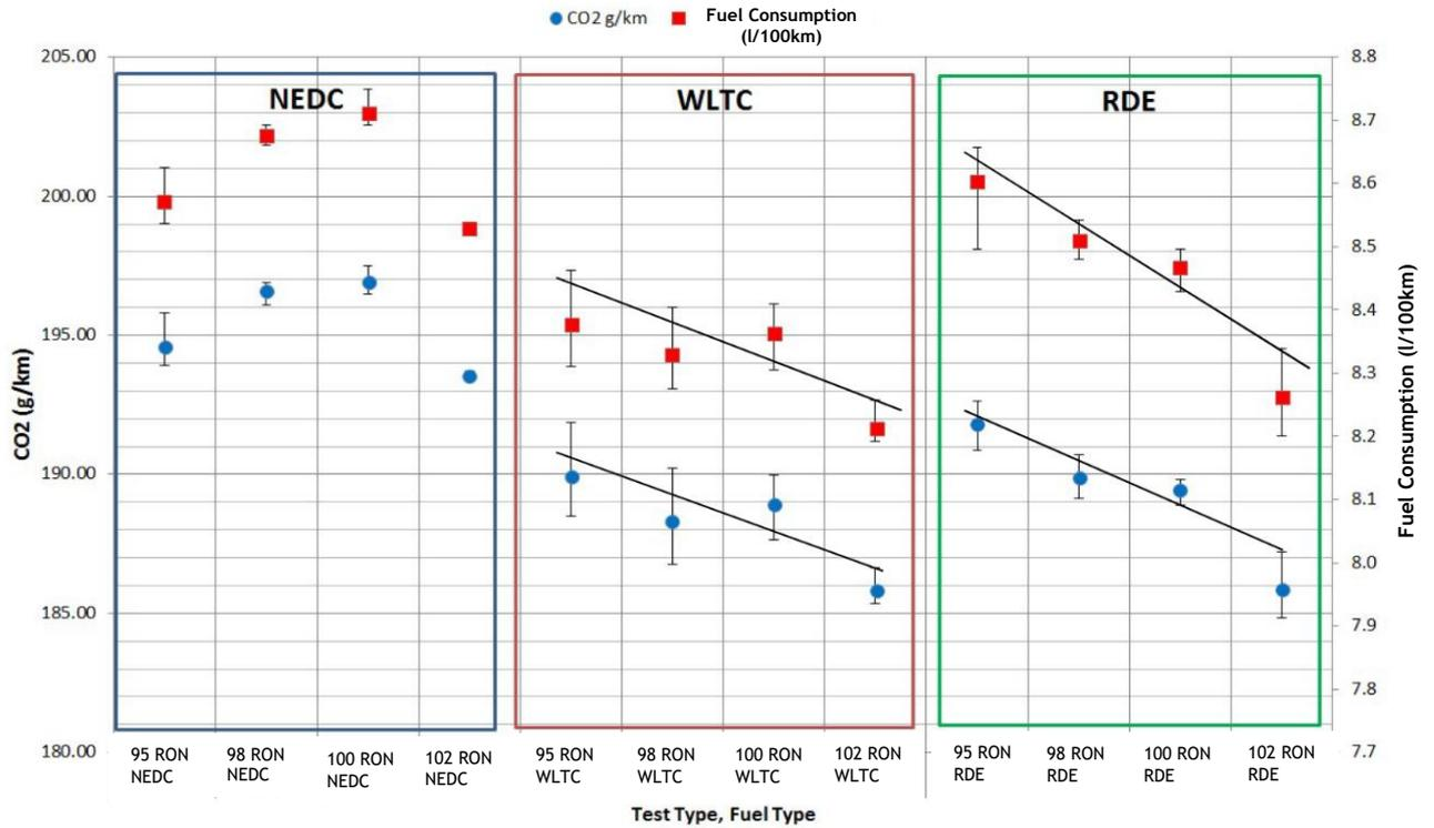
Figure 16. Averaged CO<sub>2</sub> and Fuel Consumption results for measured test cycles
