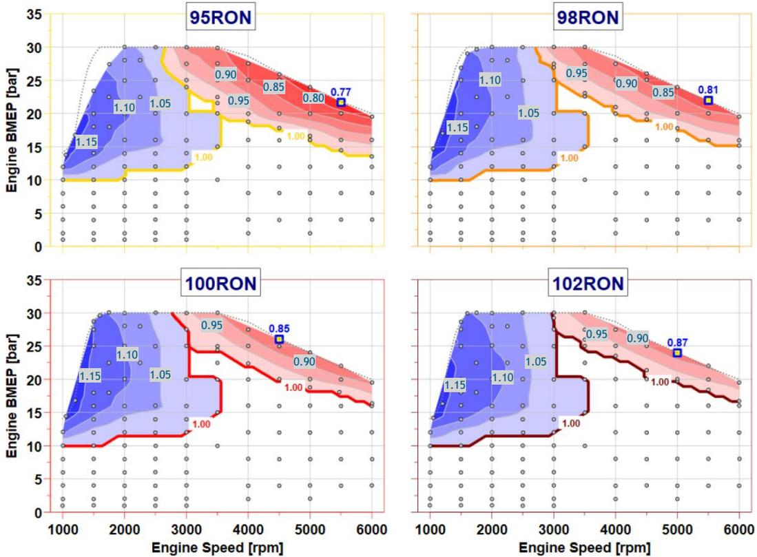
Figure 12. Contour plots for over-fuelling and under-fuelling
