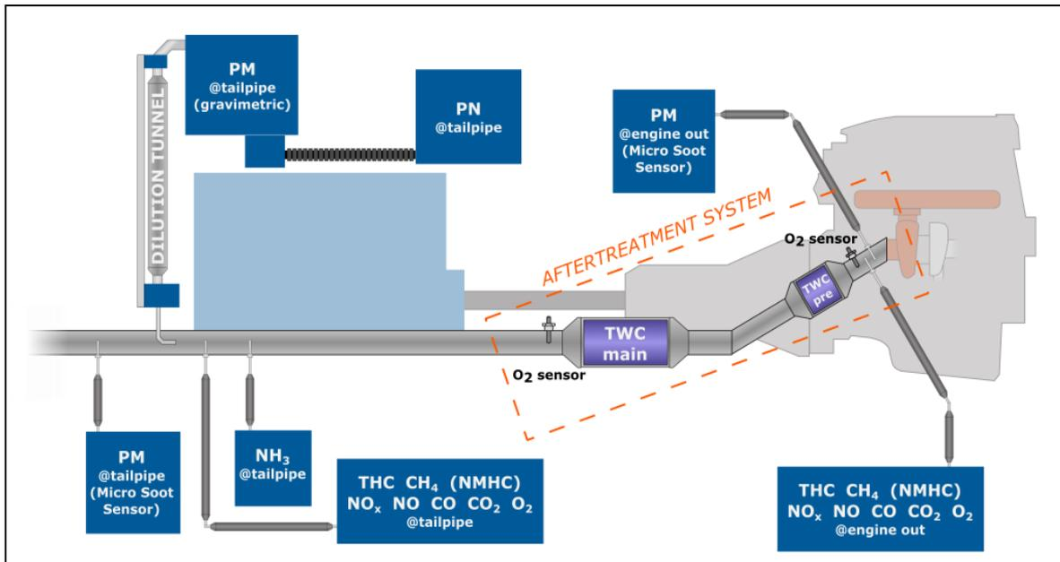
This setup was used for both engine dyno test cycles performed in this study: Worldwide Harmonized Test Cycle (WHTC) and Worldwide Harmonized Stationary Cycle (WHSC).
