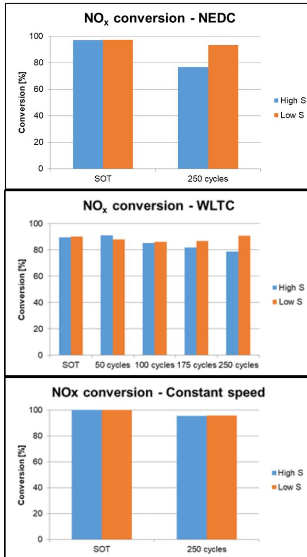
Thus, for both TWCs 50 ageing cycles appeared to complete the degreening process of the TWC regarding elimination of NO<sub>x</sub> - performance was better than that point than at 0 cycles. Thereafter, the High S TWC's performance deteriorated monotonically. The Low S TWC appeared to undergo at least two counteracting processes, which caused fluctuations in its efficiency over the WLTC at with better performance following 250 cycles than following 100 or 175.
