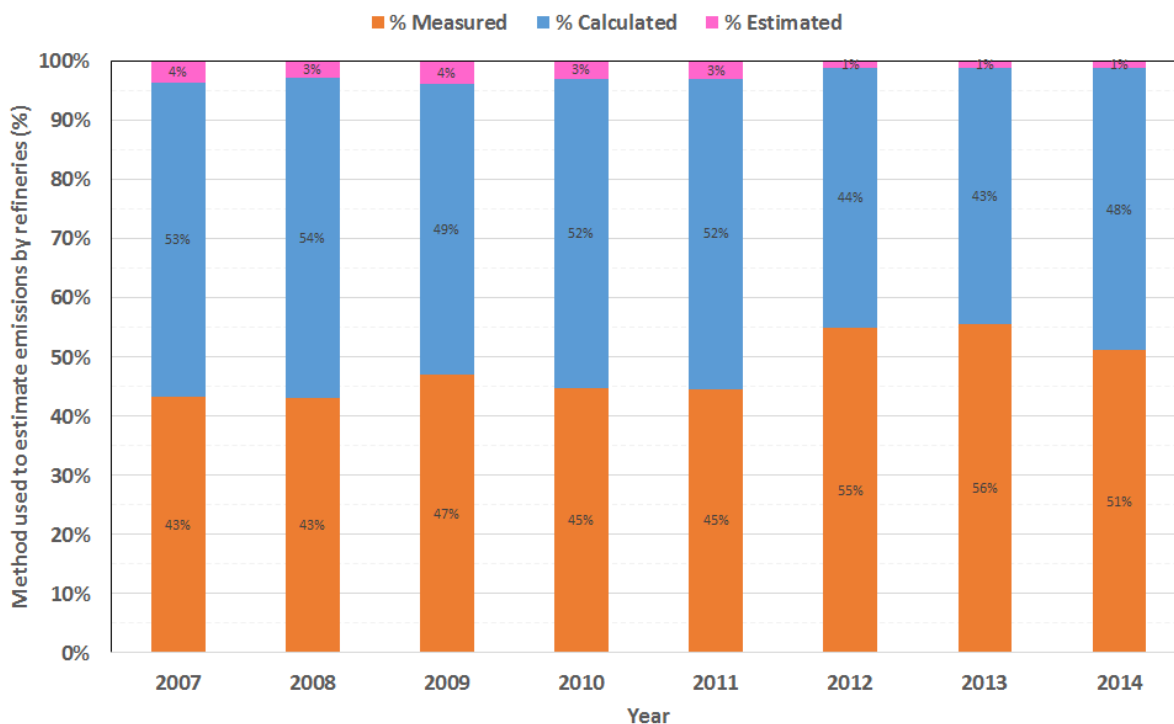
Figure 5 Methods used to determine oxides of sulphur air emissions for European refineries.
