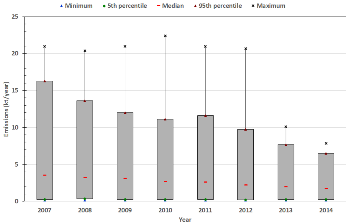
Figure 4 Statistical analysis of oxides of sulphur air emissions for European refineries: 5 th and 95 th percentiles.
