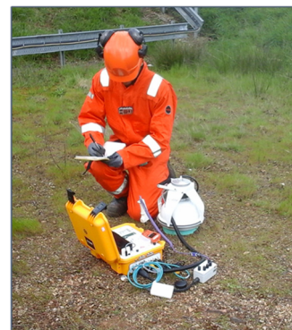
Figure 5: Field measurement using DCC method (using Licor LI-8100A) .
