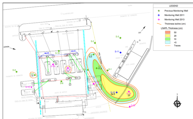
Figure 3: Thickness of the LNAPL plume, May 2014.
