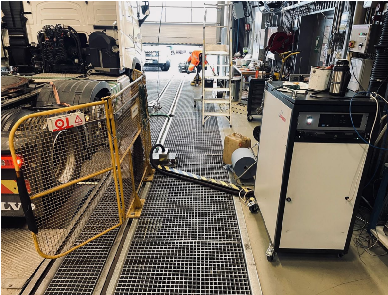
Figure 5-7 FTIR connected to the exhaust line of the test vehicle.
