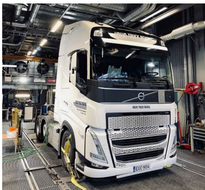
Figure 5-3: The test vehicle on the heavy-duty chassis dynamometer.
