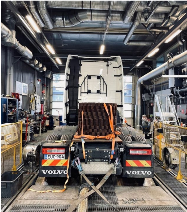
Figure 5-4: A rear-view of the test vehicle installed on the heavy-duty chassis dynamometer.
