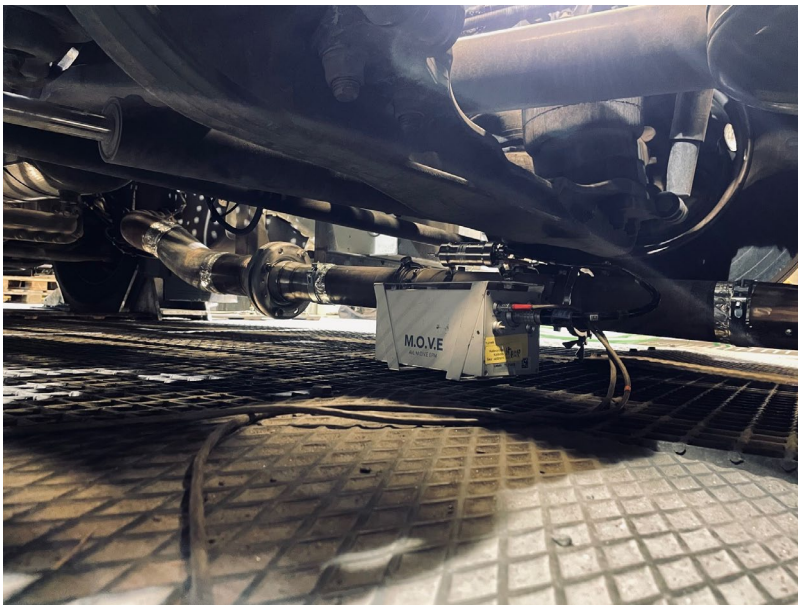
Figure 5-8 Exhaust line connected to the exhaust flow meter (EFM).
