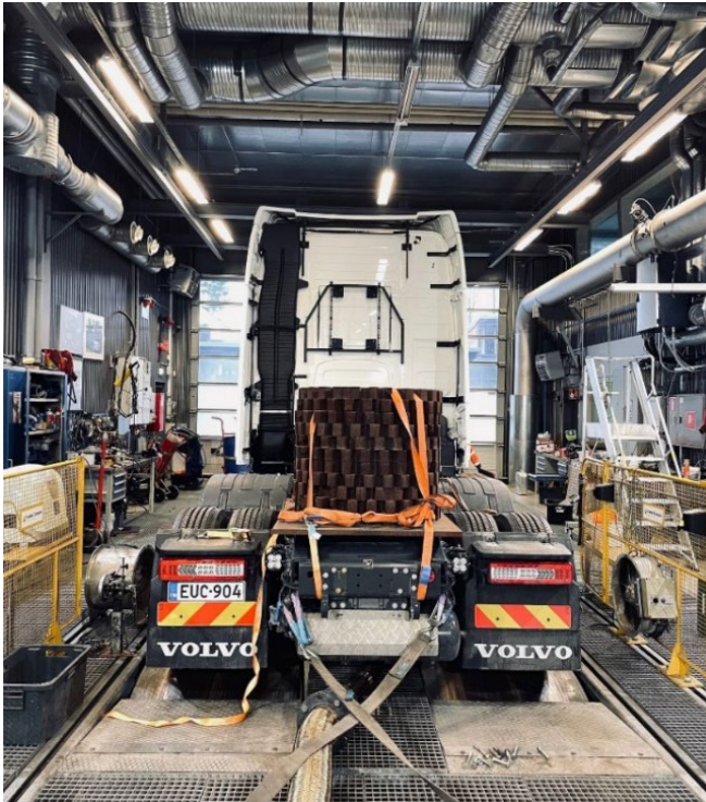
Figure 5-4: A rear-view of the test vehicle installed on the heavy-duty chassis dynamometer.
