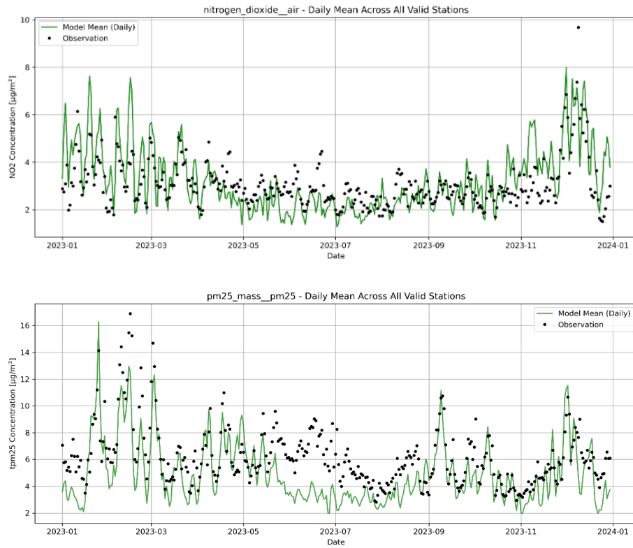
Figure 9 Daily average modelled (line) and EBAS observed (points) concentrations of \text{NO}_2 (top) and \text{PM}_{2.5} (bottom) in the EU domain for 2023
