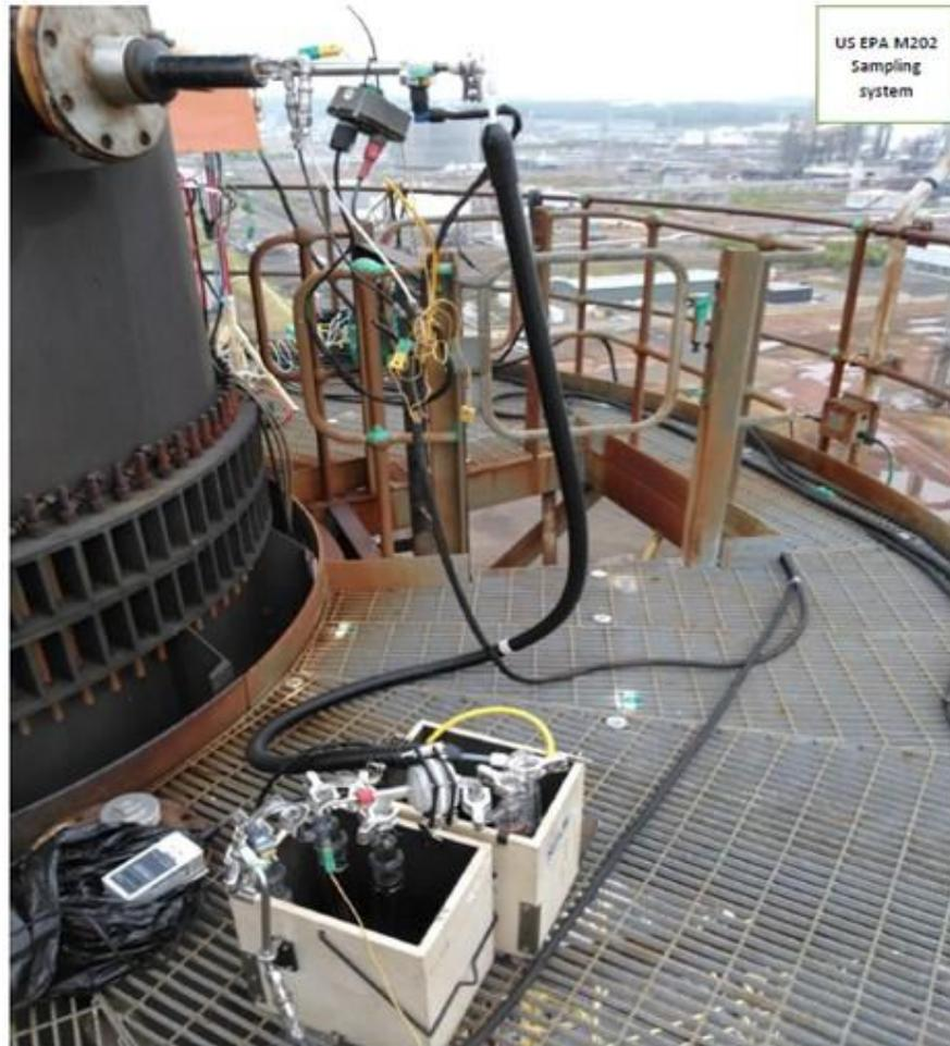
**Figure A1.3** The US EPA M202 sampling system installed on heater stack.
