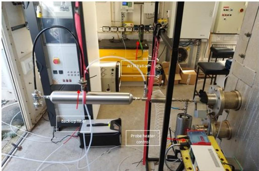
**Figure A1.1** The Dekati modified Deed-300 Dilution sampling system installed on stack simulator at NPL's laboratory.
