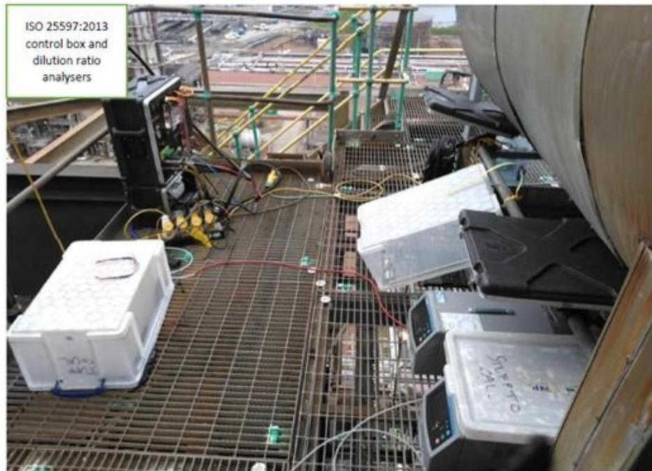
**Figure A1.2** The Dekati modified Deed-300 Dilution sampling system installed on heater stack.
