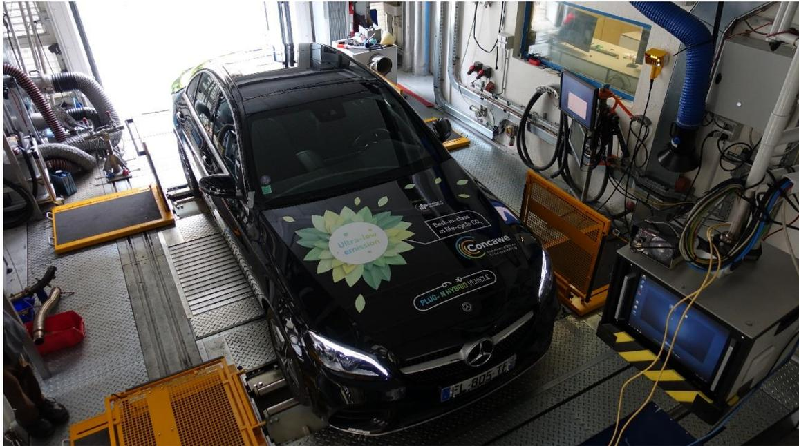
**Figure 2** Picture of the chassis dyno setup with the tested vehicle
