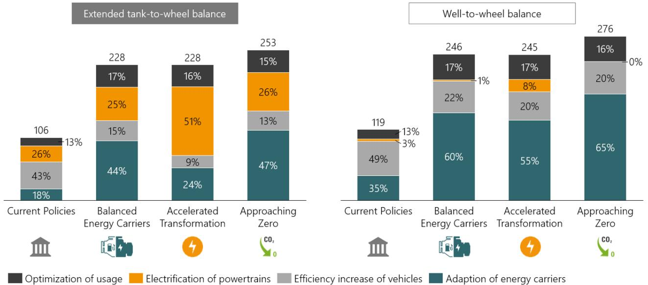
Figure 2: Comparison of the CO<sub>2</sub> emission reduction in million tons in the four scenarios and breakdown by the four measures in the extended tank-to-wheel balance (left) and the well-to-wheel balance (right) by 2050 compared to 1990.
