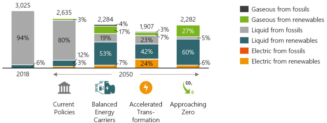
Figure 3: Final energy demand of heavy-duty trucks in Europe in PJ, shown by energy carrier type and source in 2018 and 2050 in the four scenarios. The final energy demand does not include the energy to process the energy carriers.
