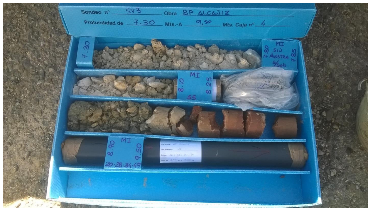
Photo 16. SV3 core box 7,30 m to 9,50 m.
