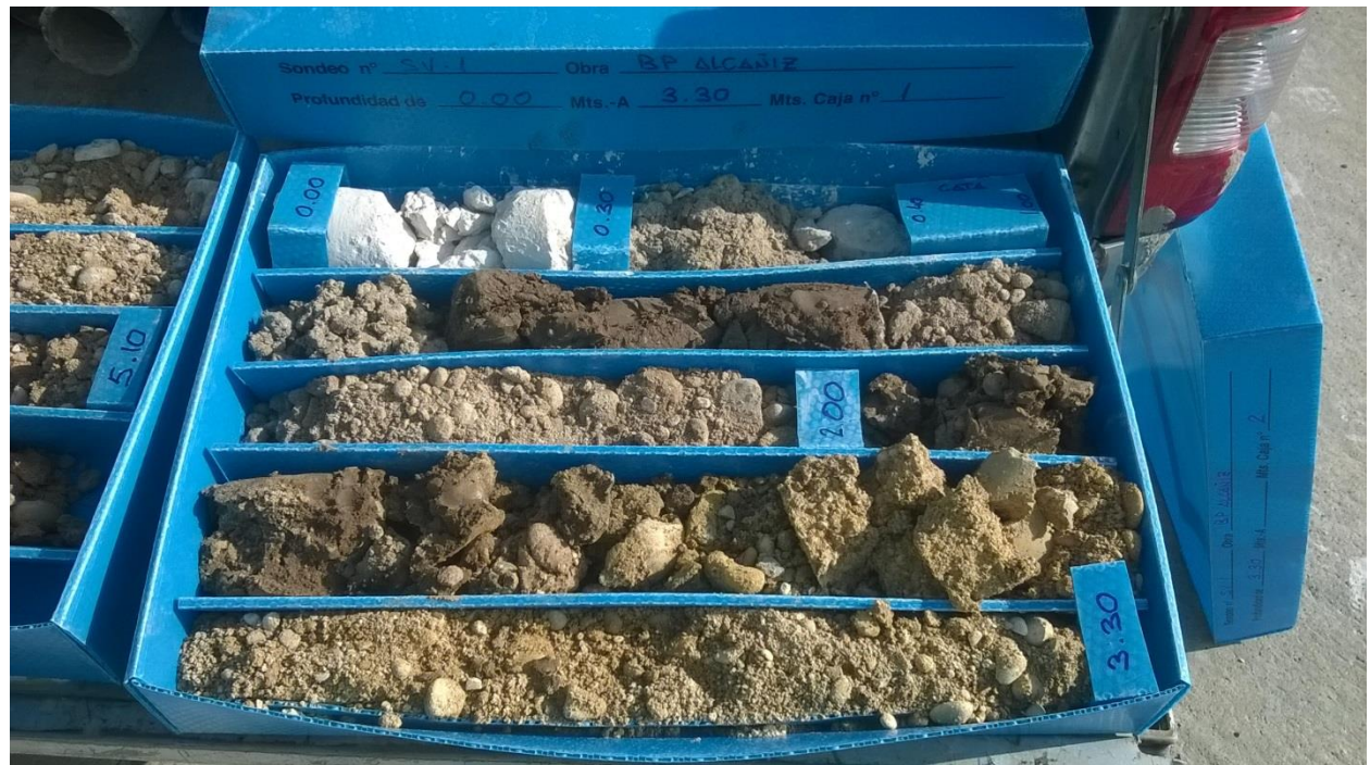
Photo 3. SV1 core box 0,0 m to 3,30 m.
