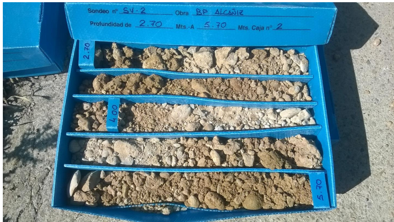
Photo 9. SV2 core box 2,70 m to 5,70 m.
