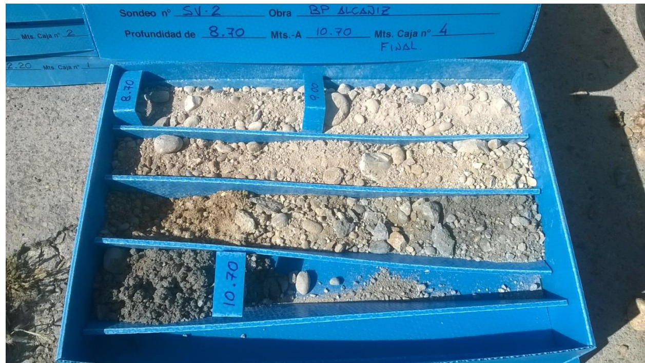
Photo 11. SV2 core box 8,70 m to 10,70 m.
