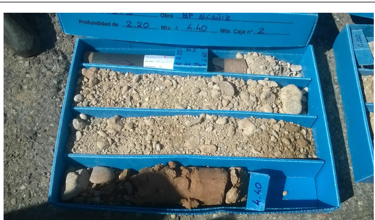
Photo 14. SV3 core box 2,20 m to 4,40 m.
