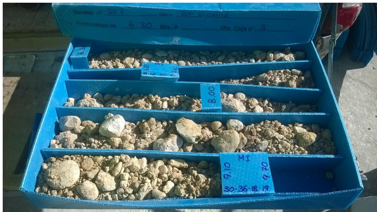
Photo 6. SV1 core box 6,30 m to 9,70 m.
