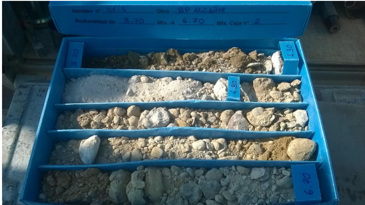
Photo 19. SV4 core box 3,70 m to 6,70 m.
