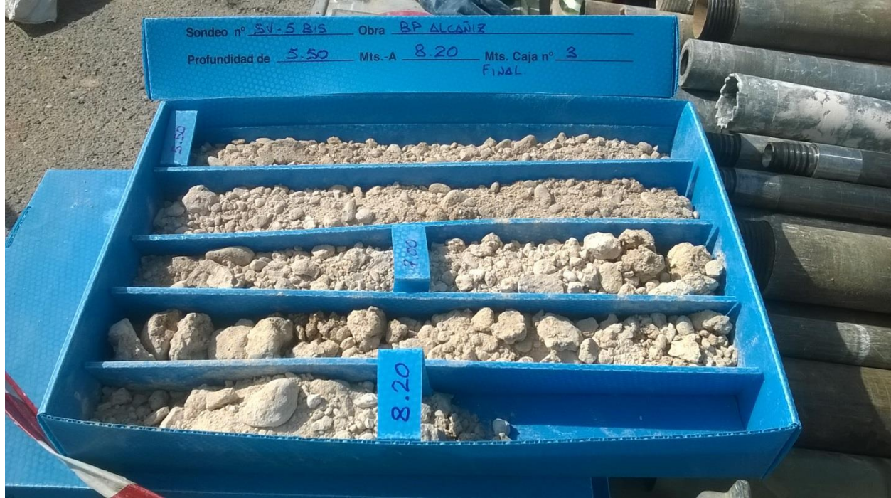
Photo 29. SV5 core box 5,50 m to 8,20 m.
