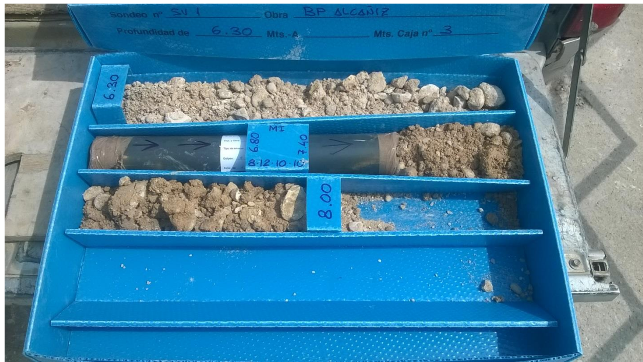
Photo 5. SV1 core box 6,30 m to 8,0 m.
