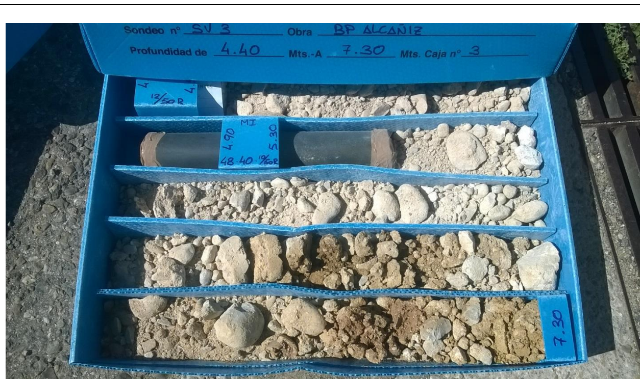
Photo 15. SV3 core box 4,40 m to 7,30m.
