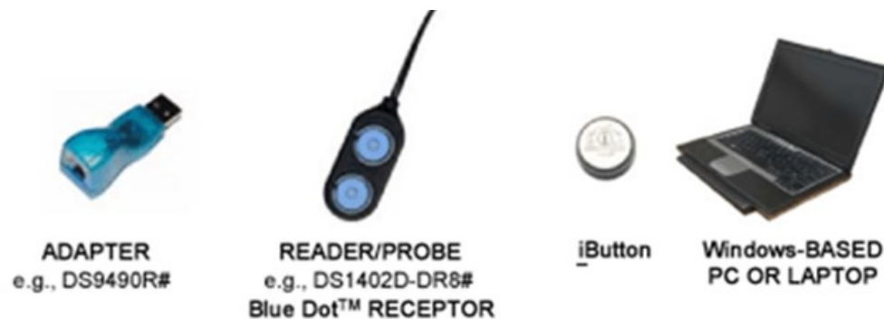
Figure 9: Components needed to program the ibutton temperature sensor.
