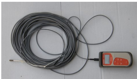
Figure 6a: Thermistor at the end of a data cable that is marked at one foot intervals and weighted (with a stainless steel bolt in the picture) below the thermistor for long cables (>25 feet).
