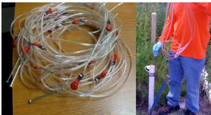
Figure 11. (a on left) string of ibuttons prepared at 2 foot intervals; (b on right) string of ibuttons lowered into a well.
