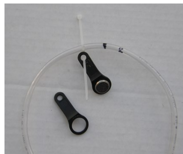
Figure 6b: Sensors (ibuttons) placed in a rubber holder and attached with plastic ties to tygon tubing marked at discrete depths.
