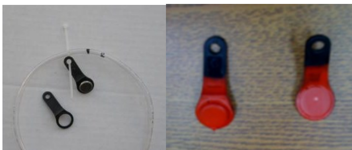
Figure 10: (a on left) shows key ring holder and ibutton as attached to tygon tubing; (b on right) waterproofed ibuttons.
