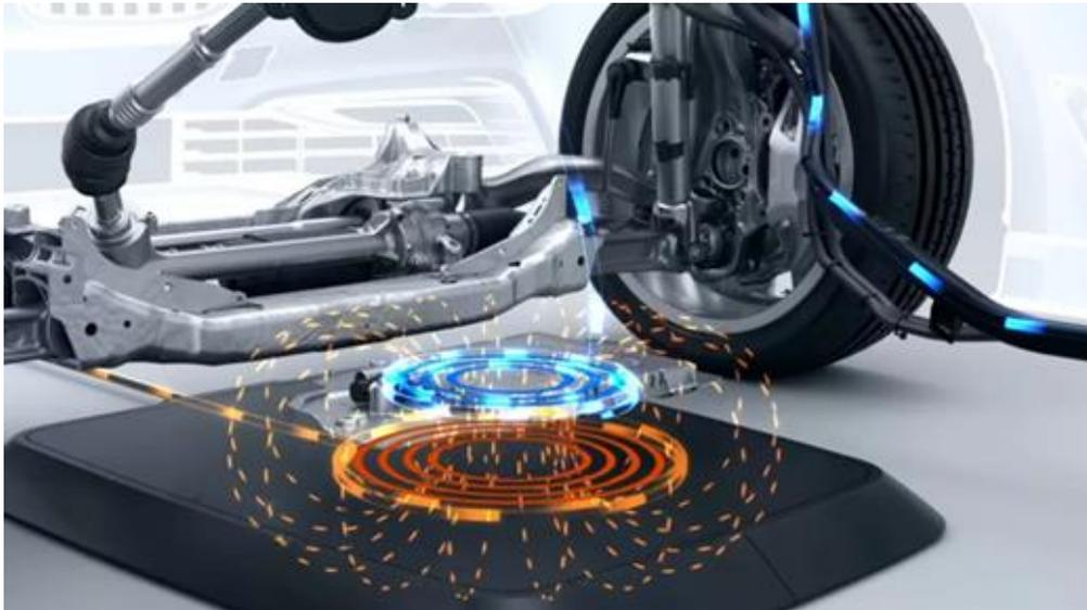
Figure 41. Illustration of the inductive (wireless) charging principle
