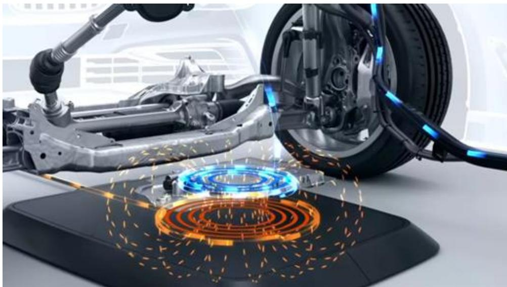
Figure 41. Illustration of the inductive (wireless) charging principle
