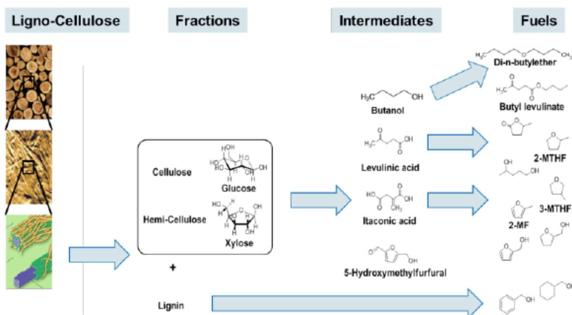
Figure 13. Possible production pathways for tailor-made fuels. Source [2.9]
