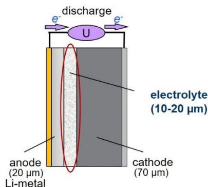
Figure 35. Scheme of one concept of a solid-state cell
