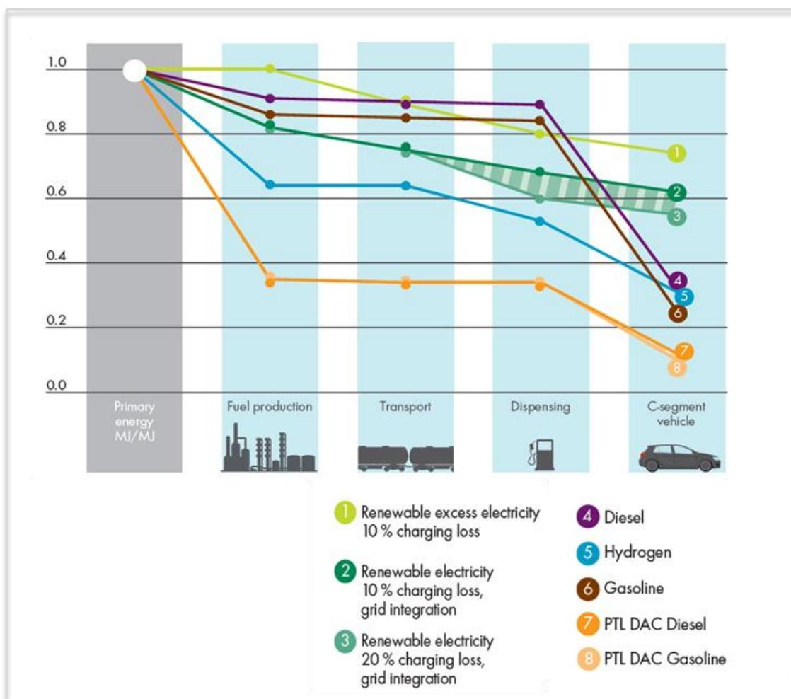
Figure 24. The Well-To-Wheel efficiency of various fuel and powertrain combinations. Source [2.15]
