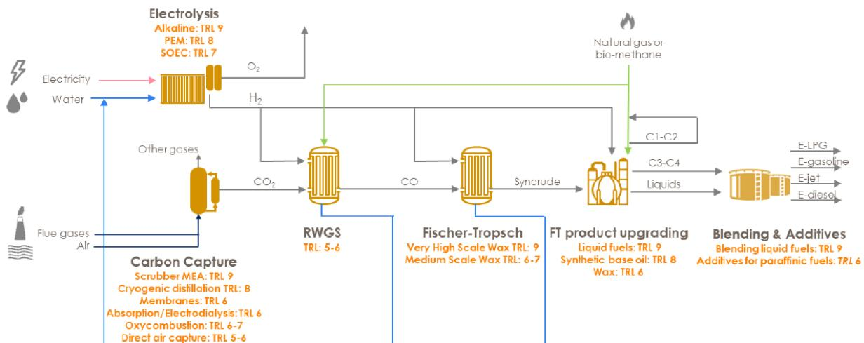
Figure 58. Summary of TRL of processes for an e-fuel synthesis via Reverse Water Gas Shift and Fischer-Tropsch<sup>108</sup>.
