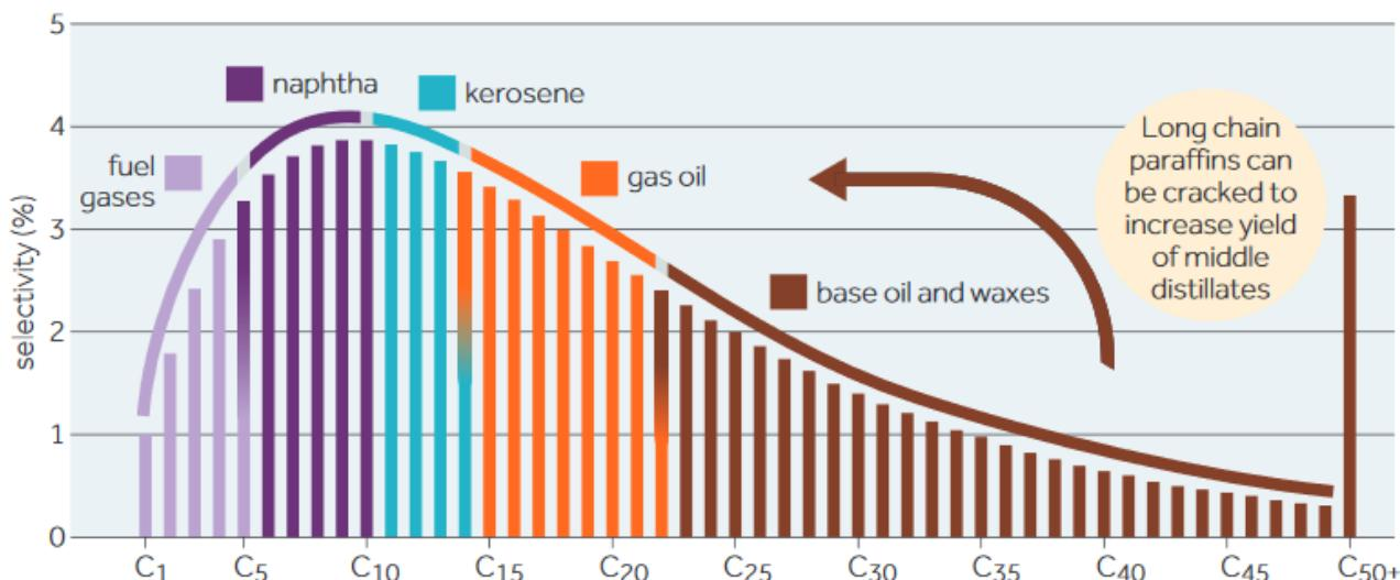
Figure 22. Fischer-Tropsch liquid e-fuel products. Source [2.15]
