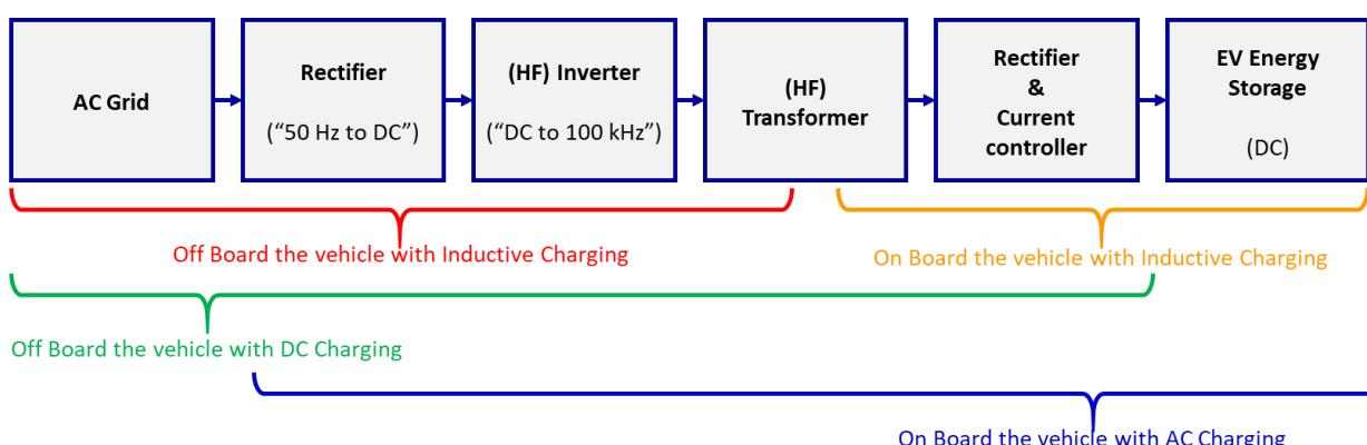
Figure 39. The functional block diagram of a generalized charger
