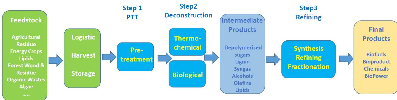
Figure 12. The main stages of biofuel production
