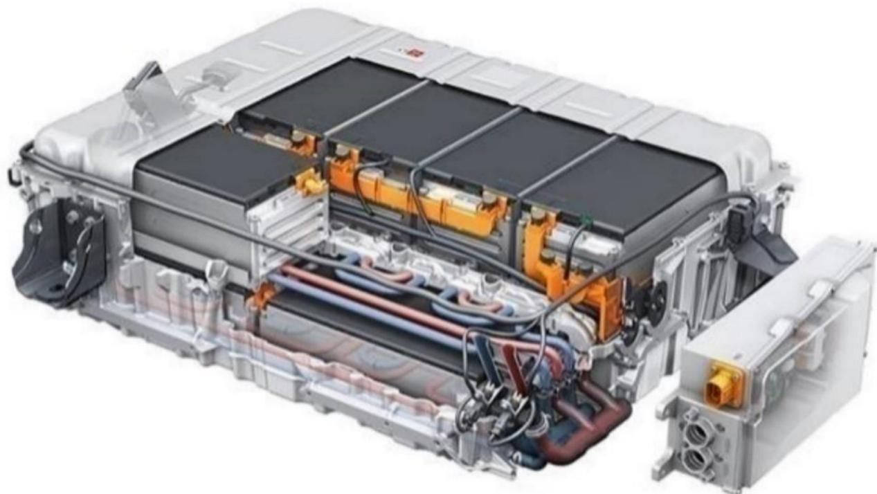
Figure 37. PC battery system with TMS (Source: Audi (website homepage))
