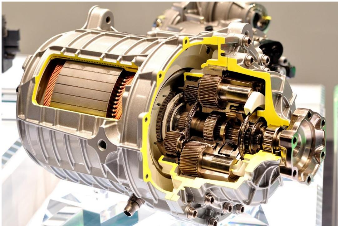
Figure 31. Integrated electric drive module
