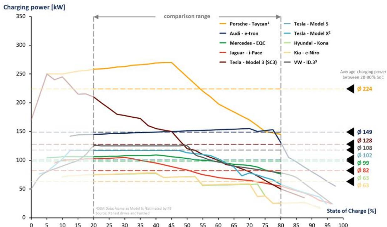
Figure 42. The different charging profiles from different BEV models (P3 study)
