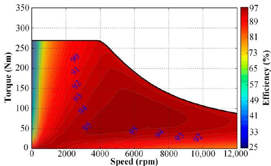
Figure 32. Typical permanent magnet synchronous traction machine (BMW i3)<sup>48</sup>
