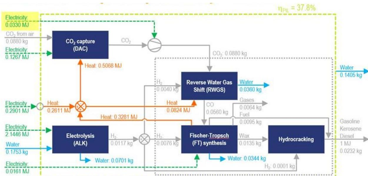
Figure 23. Resources required for liquid e-fuel production (e-Fischer-Tropsch pathway)<sup>29</sup>
