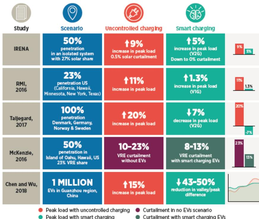
Figure 48. Smart charging for electric vehicles (IRENA: Examples of studies assessing the impact of EV charging strategies (Figure 34)). Source [4.7]
