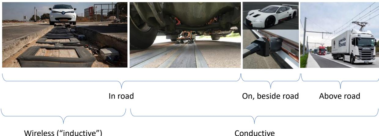
Figure 43. Different electric road system configurations and demonstration
