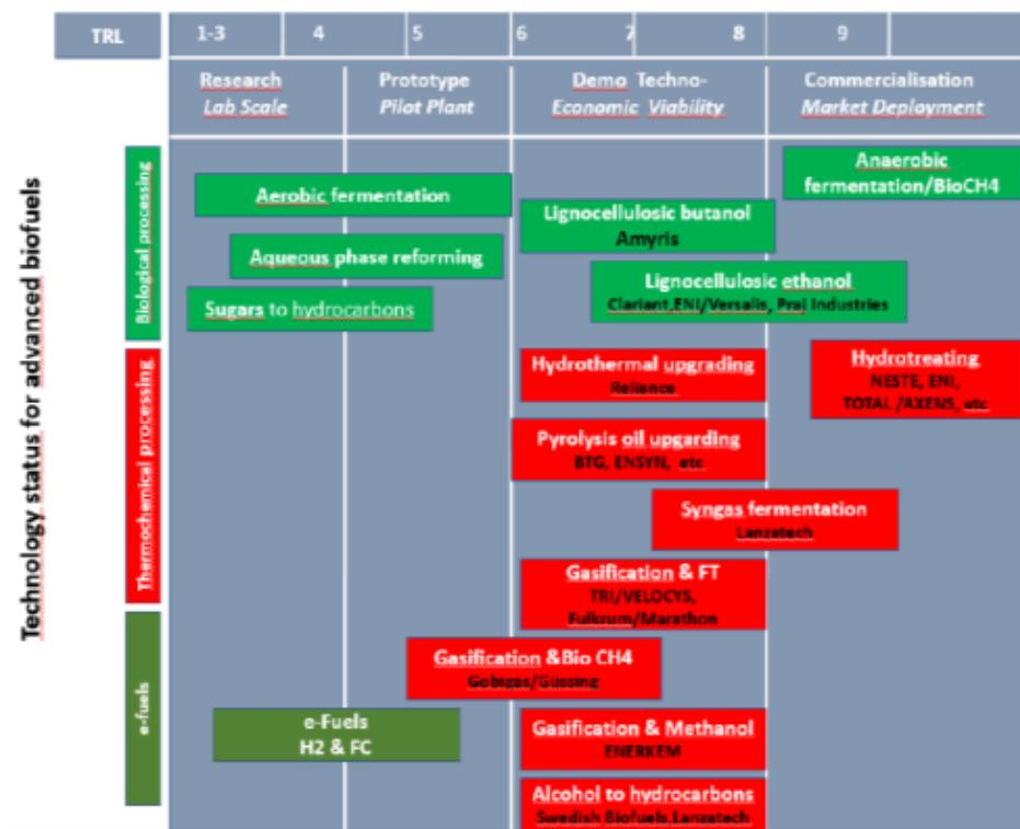
Figure 20. Advanced Fuels Conversion Technologies. Sources [2.10 & 2.11]
