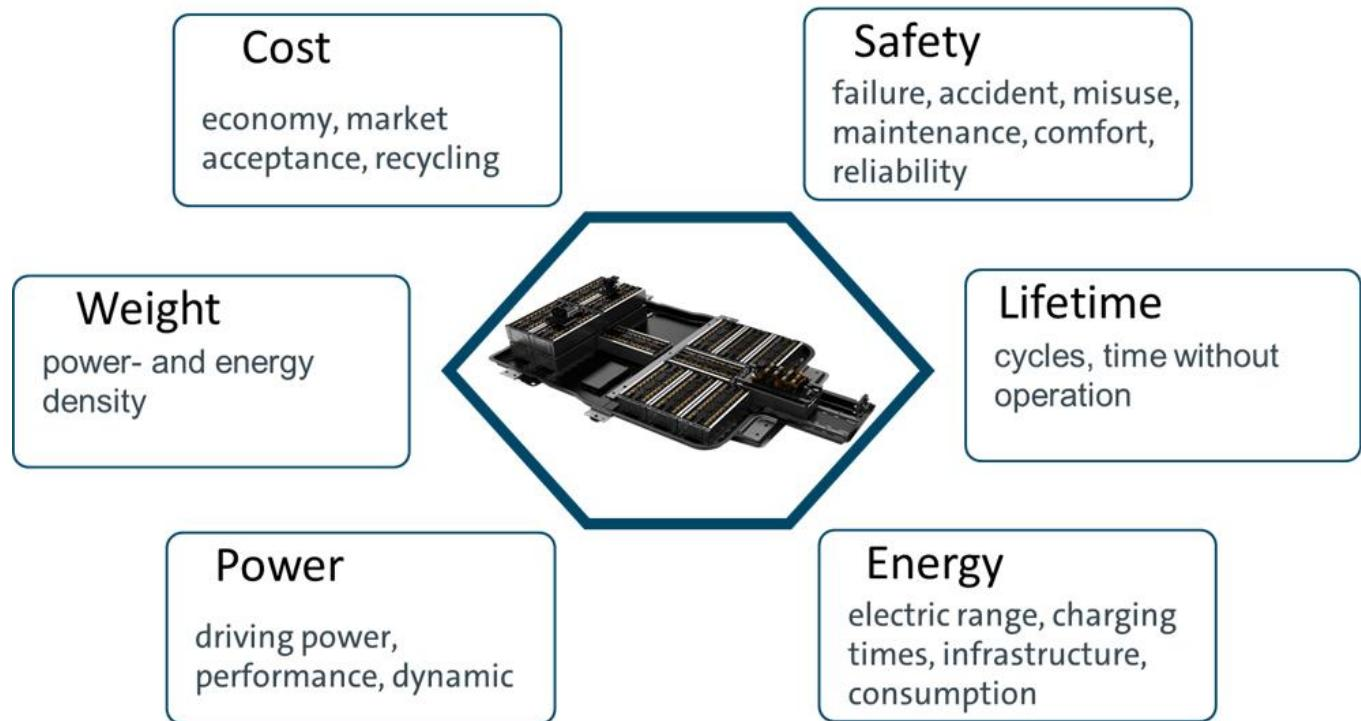
Figure 33. Requirements for batteries in road transport
