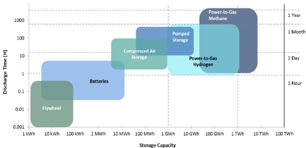
Figure 6. An overview of different energy storage technologies. Source [2.3]
