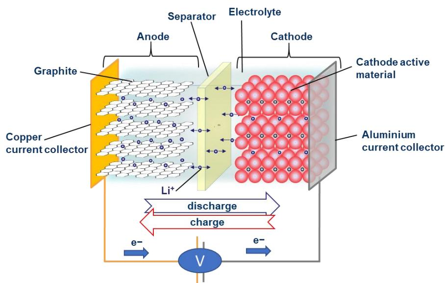
Figure 34. Structure of a Li-ion cell
