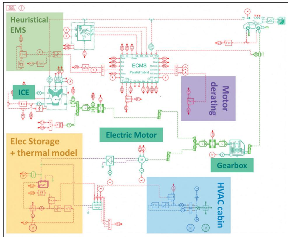
A component dedicated to hybrid architectures (ECMS: Equivalent Consumption Minimisation Strategy) was used to determine the optimal management strategy for internal combustion and electrical energy to minimise fuel consumption. It was calibrated to fit the experimental behaviour characterised on pages 18 and 19, as illustrated in Figures 6 and 7 on page 21.
