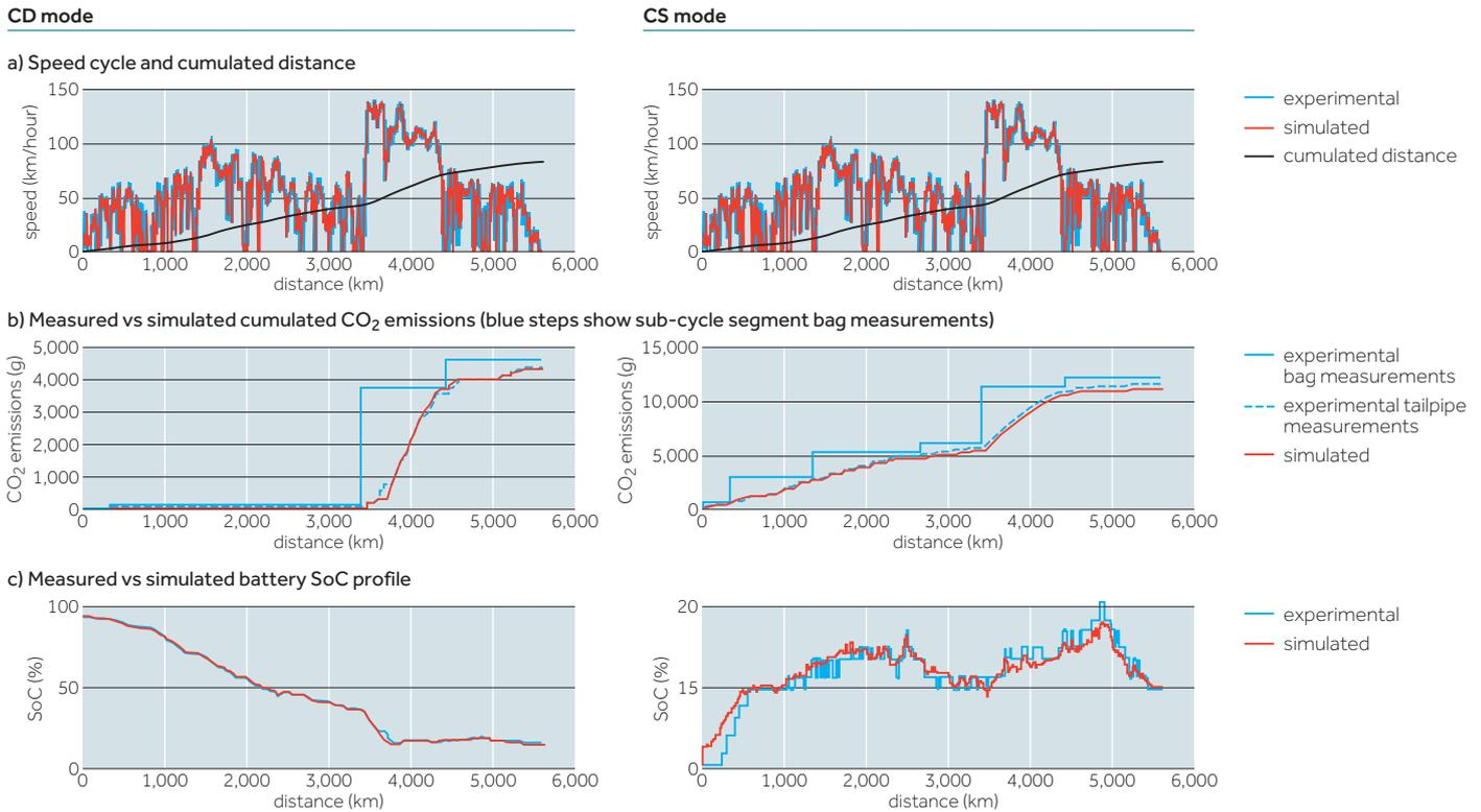
Figure 7: Comparison between the experimental and simulation results for the gasoline and diesel PHEVs, in CD and CS modes
