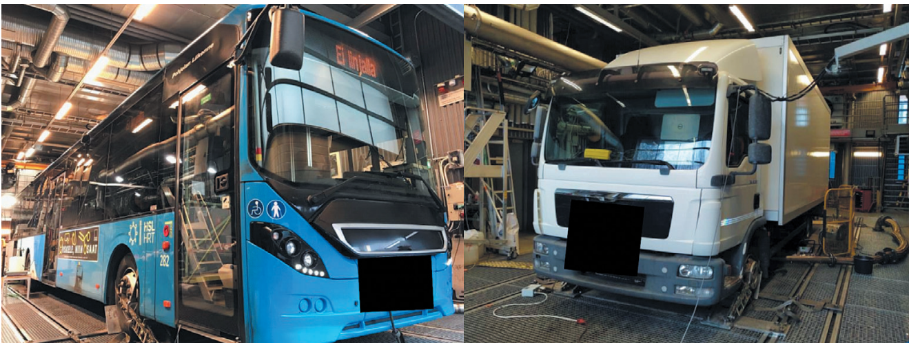
Figure 2: Commercial vehicles on a chassis dynamometer
