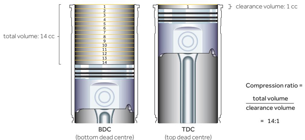
Compression ratio is calculated by dividing the total volume of the cylinder when the piston is at BDC by the clearance volume when the piston is at TDC. In the example on the right, the compression ratio would be expressed as 14:1.
