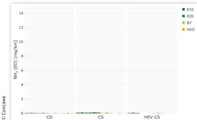
**FIGURE 36** Comparison of Tailpipe NH<sub>3</sub> emissions [mg/km] measured on RDE cycles on chassis dyno for each fuel and mode.
