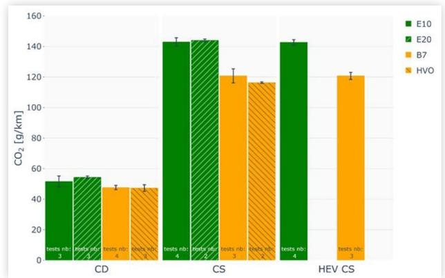
**FIGURE 16** Comparison of corrected tailpipe CO<sub>2</sub> emissions [g/km] measured on RDE cycles on chassis dyno for each fuel and mode.
