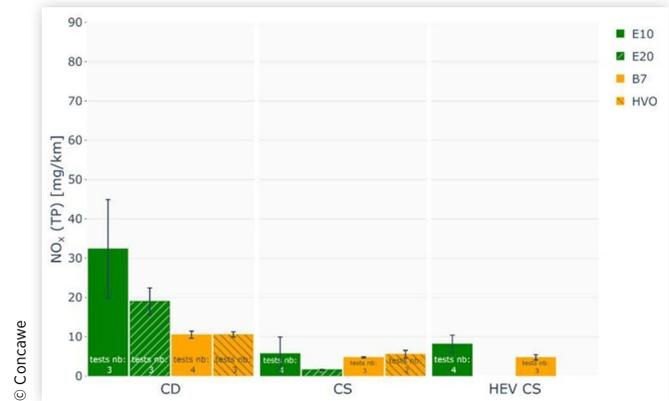
demonstrates high conversion efficiencies, over 95% in CS mode, as shown in Figure 19. Despite higher engine-out NOx emissions, E20 shows lower tailpipe NOx compared to E10 in CD and in CS, de facto improving the AFTS conversion efficiency. HVO does not impact NOx AFTS conversion efficiency compared to B7, nor does HEV compared to PHEV.
