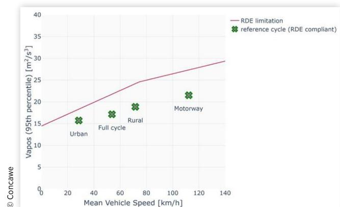
**FIGURE 5** Relative Positive Acceleration (RPA) on RDE reference cycle on roller test bench, by urban, rural, motorway phases and over the whole cycle, compared to RDE boundary.
