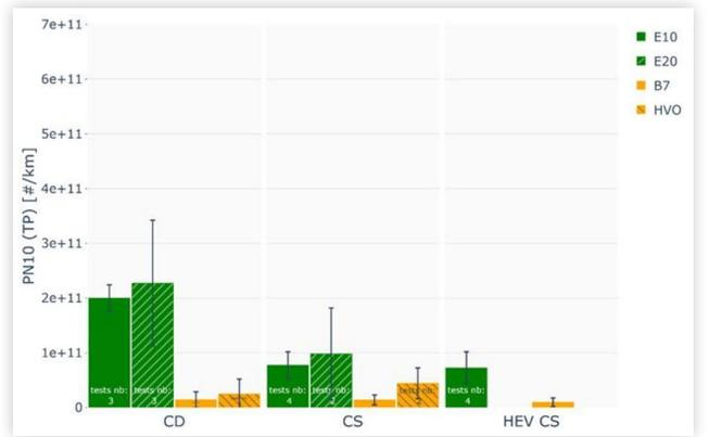
**FIGURE 21** Comparison of engine-out PN10 emissions [# /km] measured on RDE cycles on chassis dyno for each fuel and mode.
