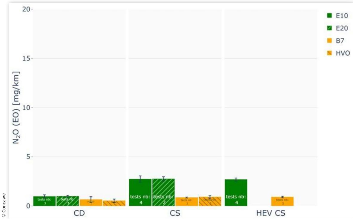
**FIGURE 50** Comparison of tailpipe  $N_2O$  emissions [mg/km] measured on RDE cycles on chassis dyno for each fuel and mode.
