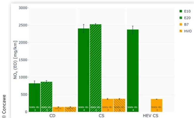
**FIGURE 18** Comparison of tailpipe NOx emissions [mg/km] measured on RDE cycles on chassis dyno for each fuel and mode.
