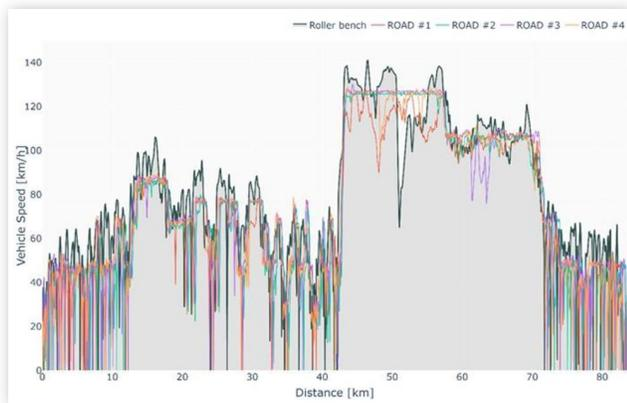
**FIGURE 8**  $V^*$  measured during on-road-tests compared to RDE boundaries.
