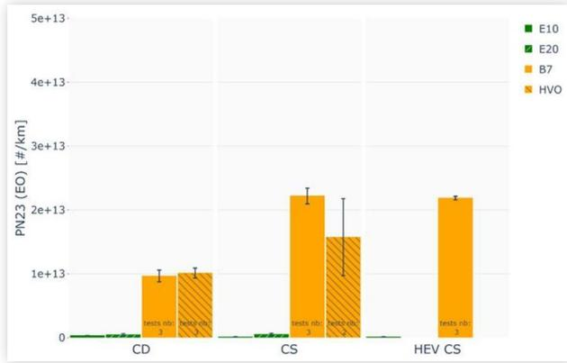
**FIGURE 22** Comparison of tailpipe PN23 emissions [# /km] measured on RDE cycles on chassis dyno for each fuel and mode.
