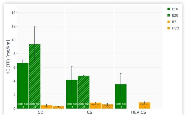
THC emissions of the Diesel PHEV fueled with B7 are 80 % lower than the ones of the gasoline PHEV fueled with E10 in CS.
