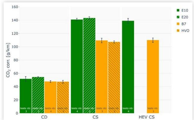
Reducing the mass of the vehicle, i.e. HEV mode, does not impact the CO<sub>2</sub> emissions, for gasoline, as well as for Diesel. Similarly to the volumetric fuel consumption, it is quite a surprising result.
