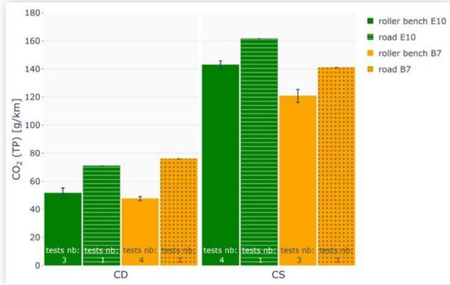
PHEV in CS (+13.5% when corrected), are observed for the on-road tests despite milder driving conditions. These gaps were assessed by using calibrated vehicle simulators (not shown in this article), and it was concluded that there was a discrepancy between the “real-world” road law and the roller test bed road law which explains the stated difference on CO<sub>2</sub> emissions.
