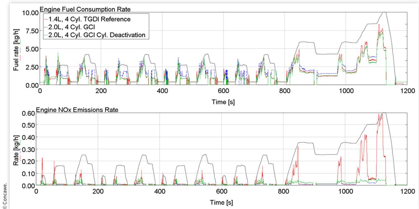
**FIGURE A3** Simulated fuel and NOx mass flow rates of different engine concepts in WLTC
