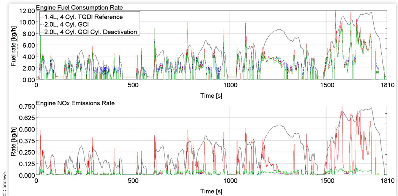
**FIGURE A4** Simulated fuel and NOx mass flow rates of different engine concepts in RDE
