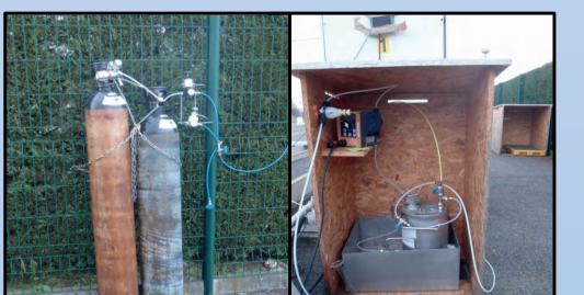
Specific equipment was used for the injection of the mixture of effluent and petroleum distillate. A mixing valve was used to improve dissolution of hydrocarbons in the water. In order to avoid volatilization of the distillate during the experiments, the headspace in the containers
