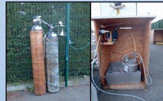
Specific equipment was used for the injection of the mixture of effluent and petroleum distillate. A mixing valve was used to improve dissolution of hydrocarbons in the water. In order to avoid volatilization of the distillate during the experiments, the headspace in the containers was filled with nitrogen.
