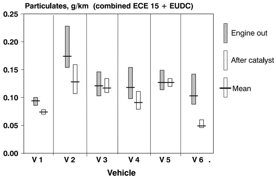
**Figure 2 Particulate emissions spread (engine out vs. after catalyst)
