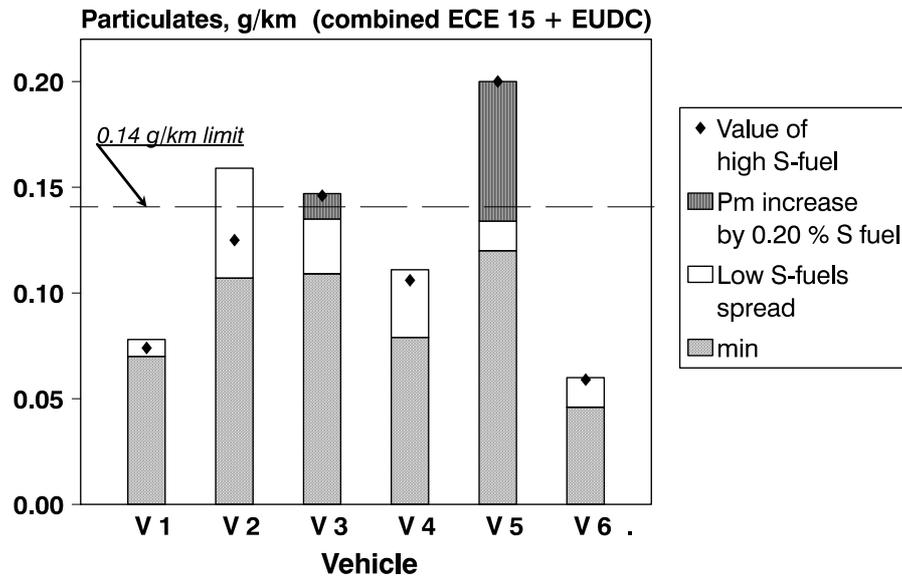
**Figure 4 Particulate emissions spread at 120 km/h const. speed, with oxidation catalyst**
