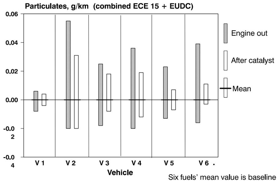
**Figure 3 Effect of fuel sulphur on particulate emissions with oxidation catalyst**
