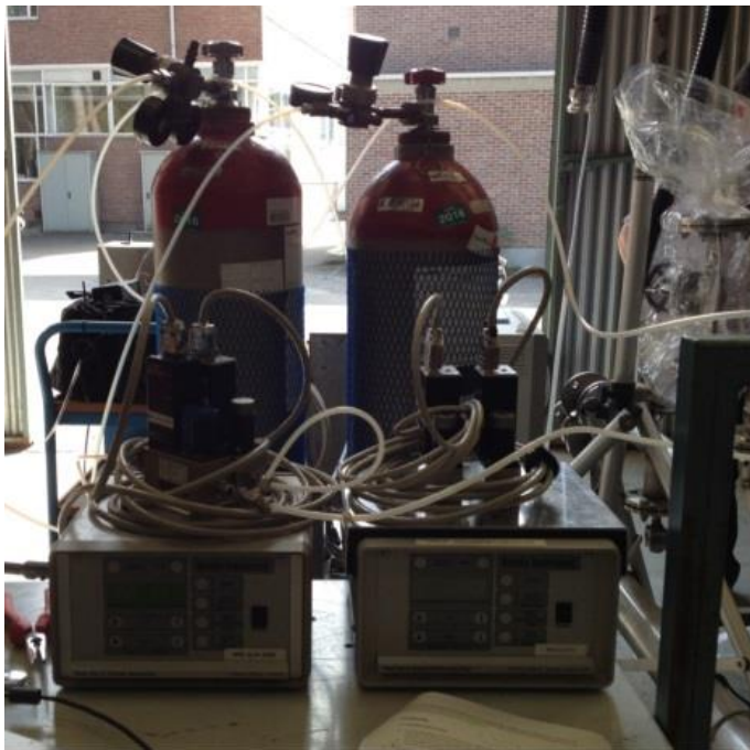
Figure 5 Mass flow controllers used during the study (Courtesy of Providence Photonics)
