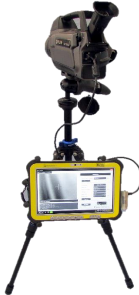
Figure 3 Set-up of QOGL system used during the study (Courtesy of Providence Photonics)
