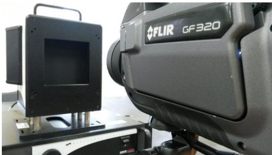
Figure 6 Synchronisation of the OGI camera with the quantification module used for the study (Courtesy of Providence Photonics)
