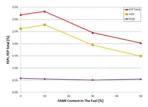
The FEP<sub>total</sub> for B10 seems to be higher compared to B0 although the difference is very small (3.3 vs. 3.2%). The higher FAME contents in the other two fuels reduce the FEP<sub>r</sub> as expected.
