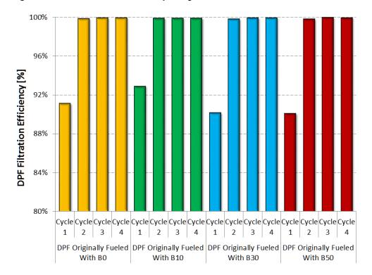
*Figure 2.* DPF filtration efficiency using market diesel fuel
