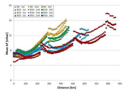
*Figure 4.* Mean NEDC pressure drop across the DPF for each fuel blend
