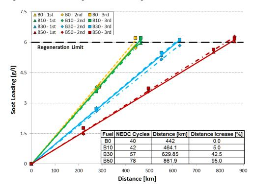
Figure 3. Soot loading based on DPF weight measurements for all fuels
