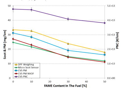
*Figure 6.* Soot and PM emissions (left axis) and particle number concentration (PNC) (right axis) versus FAME content
