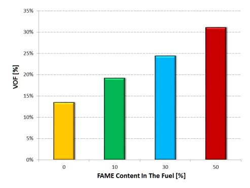
Figure 7. Volatile organic fraction (VOF) vs. FAME content
