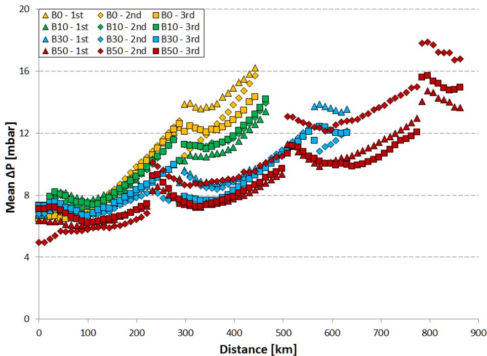
**Figure 5.** Maximum NEDC pressure drop across the DPF for each fuel blend
