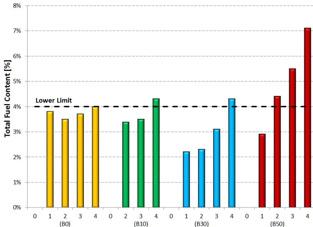
It should be noted that the dilution of engine oil with fuel should be kept below certain levels defined by the manufacturer. The recommended dilution limits range from 4-10% [22, 23, 24, 25]. Dilution levels up to 10-15% are considered to be unacceptable [26]. This indicates that this specific regeneration procedure has a significant effect on engine oil dilution with fuel. This appears to be exacerbated in the FAME containing fuels, in particular with B50 (**Figure 11**).
