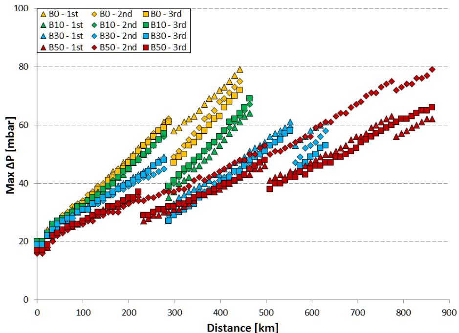
The specific PM emission measurements (without DPF) carried out after the end of the loading repetitions with all fuels provided additional information and a comparison with the results from the DPF weight measurements. The trend of decreasing PM emissions with increasing FAME content indicated by the trend in DPF weight was
