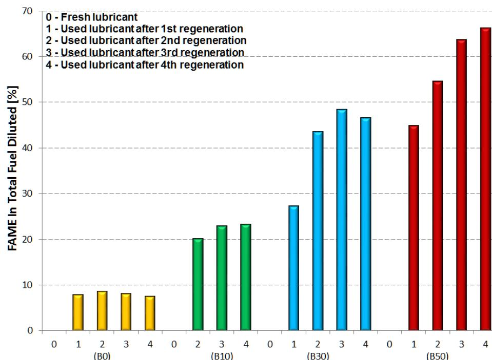
**Figure 11.** Total fuel content (DIN 51454) in the lubricant samples
