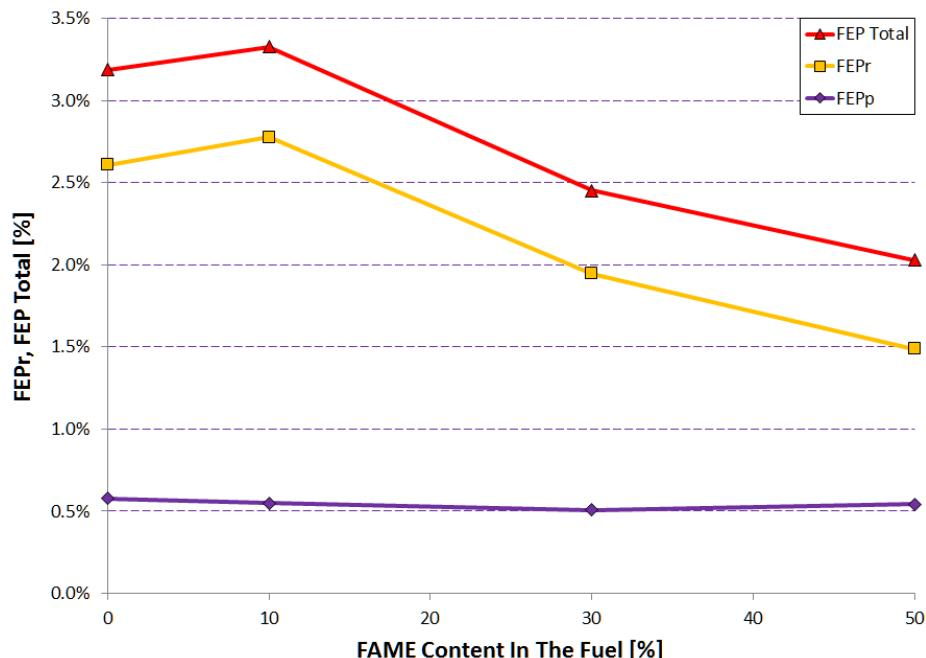
The FEP<sub>total</sub> for B10 seems to be higher compared to B0 although the difference is very small (3.3 vs. 3.2%). The higher FAME contents in the other two fuels reduce the FEP<sub>r</sub> as expected.
