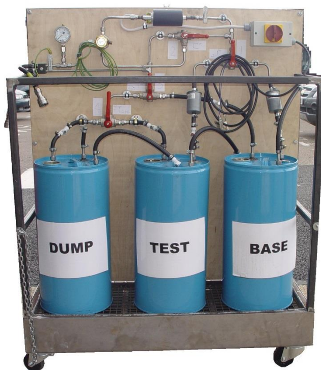
Figure 3. Fuel Changeover Rig
