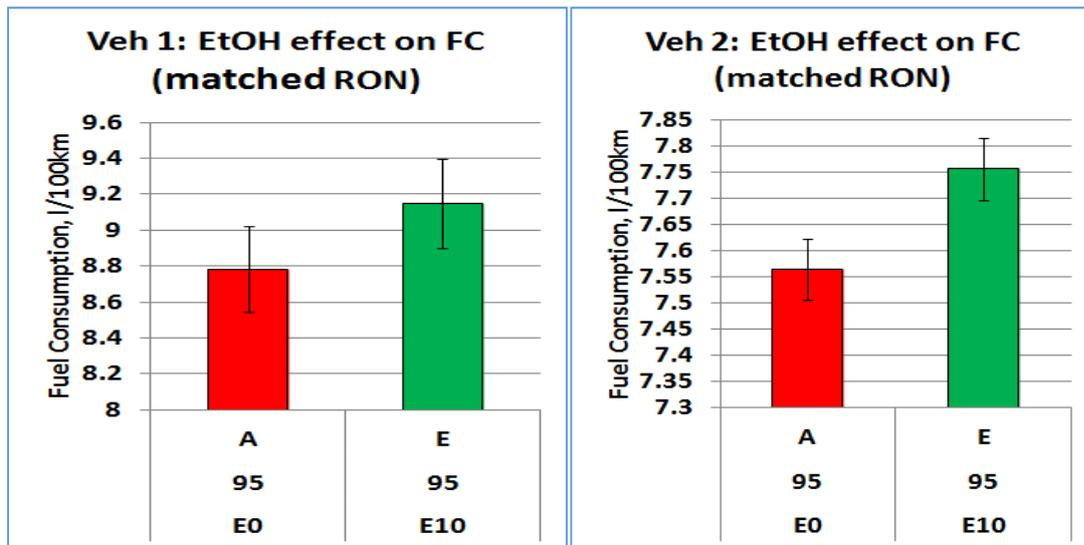
Comparison of ETBE and Ethanol containing fuels with equivalent oxygen content to 10% ethanol (**Figure 25**) gave similar increases in fuel consumption in Vehicle 2 and no significant difference in Vehicle 1.
