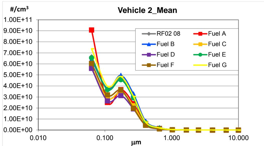
The summary histogram plot analysis of Vehicle 2 shows, **Figure 22**, the PN reduces moving from the lowest diameter, 0.063 µm to successively, 0.109 µm, 0.173 µm, and 0.267 µm. It decreases as diameter increases until the particulates disappear at over 1 µm. As reported above, the single bars represent the arithmetic mean of NEDC test repetitions run for each fuel and the error bars shown are the standard deviation calculated for the same set of values.
