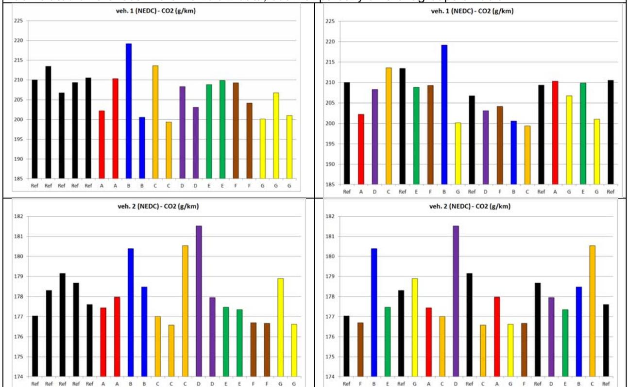
**Figure A2.6:** CO2 is somewhat variable in Vehicle 1 in particular and no fuel related trends are apparent in the data which are consistent across the vehicles.
