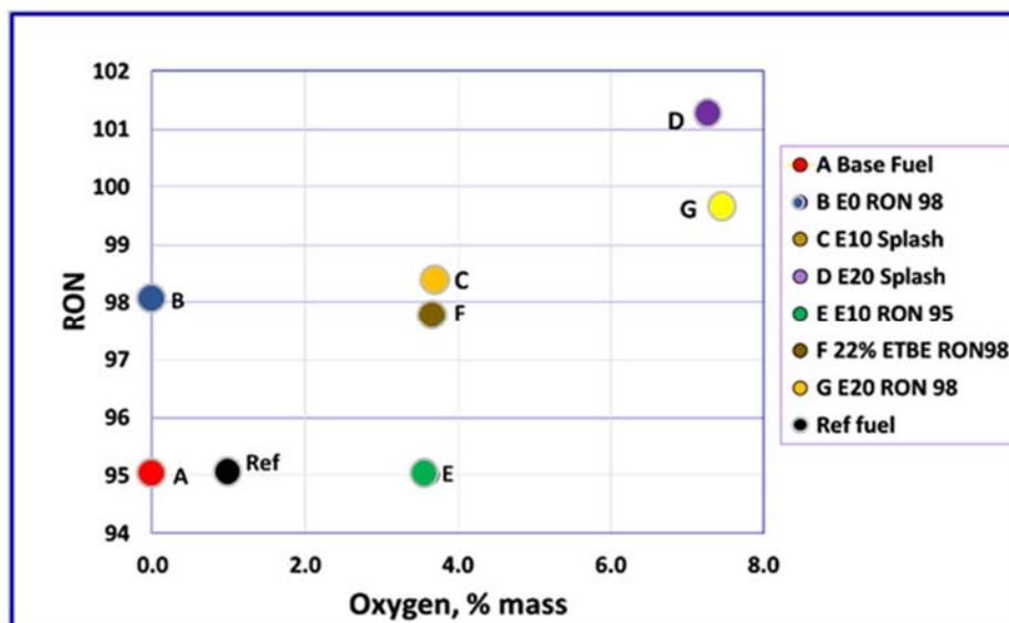
A CEC Euro 5 reference fuel was also run interspersed with the test fuels in a randomized order. The full analytical analysis of the reference fuel as well as the test fuels is given in **Appendix 6**.
