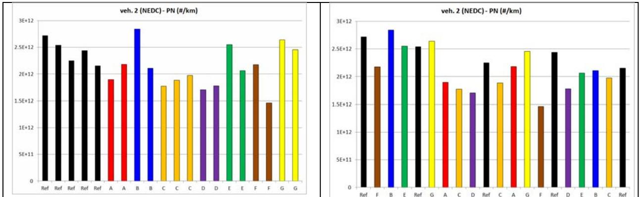
**Figure A2.5:** There is some evidence of systematic downward drift in the Vehicle 1 data over time which obscures any fuel related trends, however there are still some potential differences. There are also potential fuel related differences in the Vehicle 2 data, but with partially different groups of fuels.
