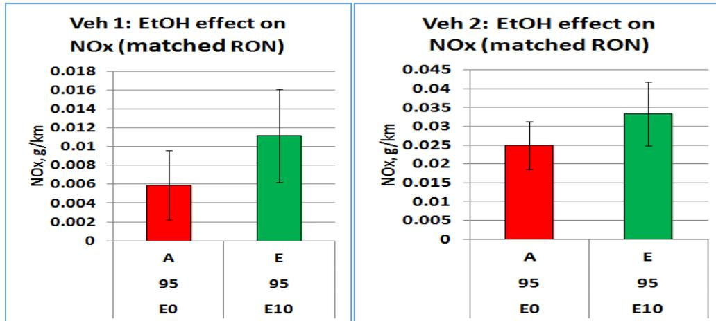
When the NOx emissions of the ETBE-containing fuel were compared with E10 with equivalent oxygen and similar RON there was no significant difference between the two in either vehicle, although in Vehicle 2, the ethanol-containing fuel showed a significant increase in NOx compared to a base without oxygenate (**Figure 31**).
