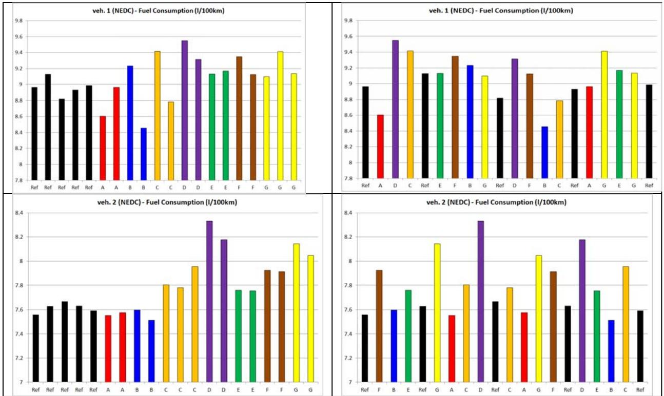
**Figure A2.7:** Fuel consumption data is noisy from Vehicle 1, but there is some evidence of higher values for higher oxygen fuels. In the Vehicle 2 data, fuel consumption is clearly higher with the higher oxygen content fuels.
