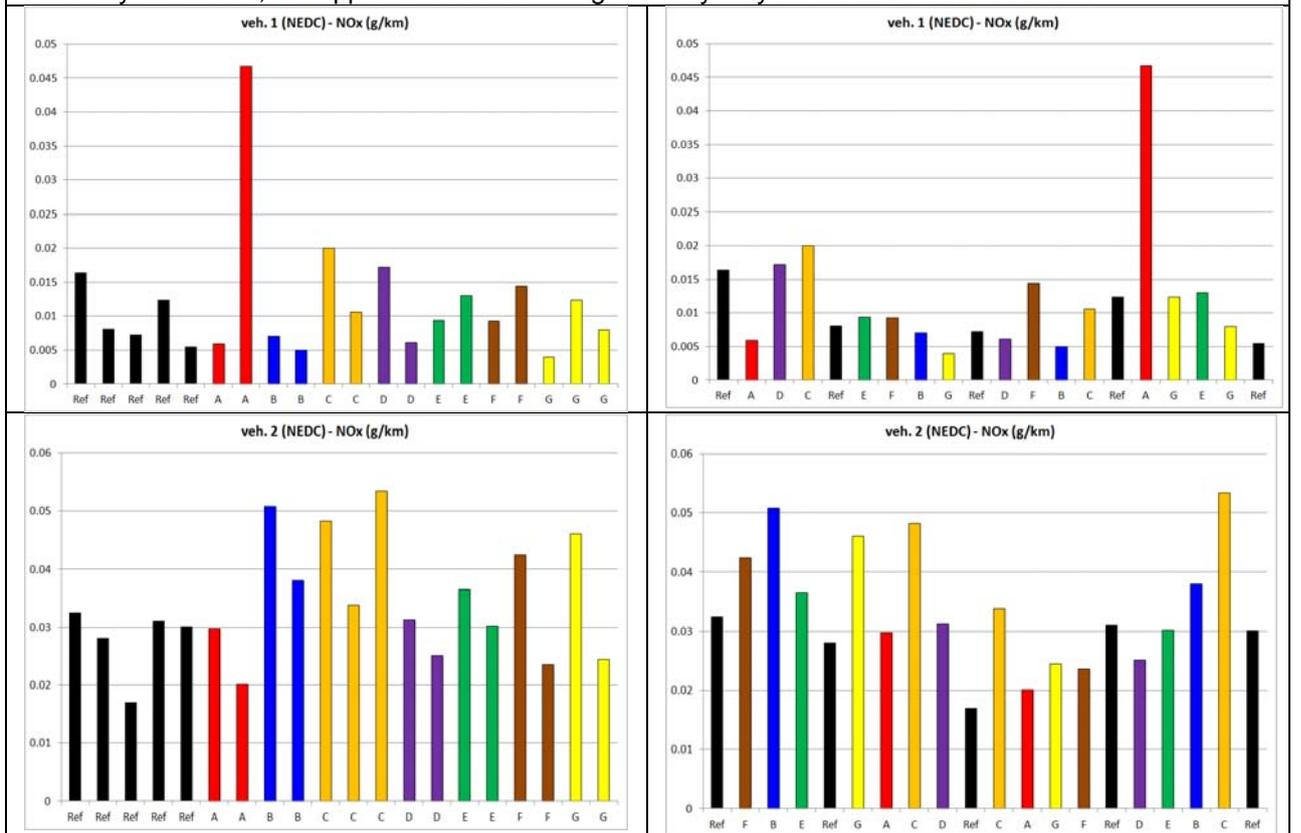
**Figure A2.3:** There is a clear high outlier in the Vehicle 1 data for the E0 base fuel which has been rejected from the main analysis as a statistical outlier. There are some potential fuel related trends in the data, though the trends are not consistent between the vehicles and therefore are questionable. There is evidence of a baseline fluctuation in the data from both vehicles over time, which would be difficult to adjust for.
