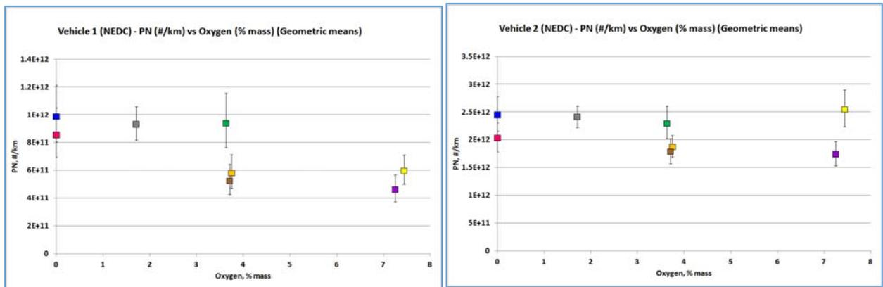
There is a statistically significant correlation between fuel oxygen content and PN at the P <5% (95%) confidence level in the Vehicle 1 data for oxygenate levels above 3.5%. This is not observed in the Vehicle 2 data. This effect is also shown below in Vehicle 1 comparing splash blended ethanol fuels at 10% and 20% ethanol (Fuels C and D respectively) with E0 (Fuel A) with no attempt to correct for RON (**Figure 13**).
