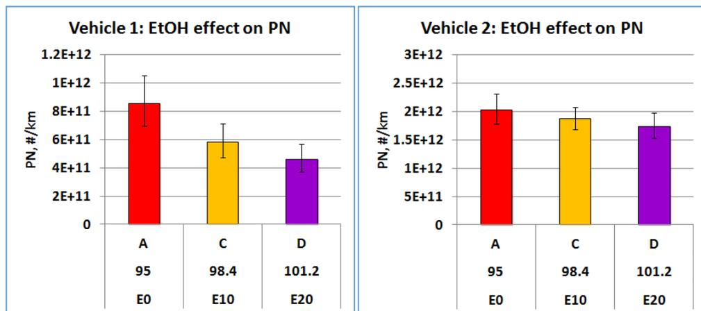
When RON is matched however there is no significant difference between non-ethanol and 10% ethanol containing fuels observed for either vehicle as shown in **Figure 14**. The error bars are overlapping in both cases.
