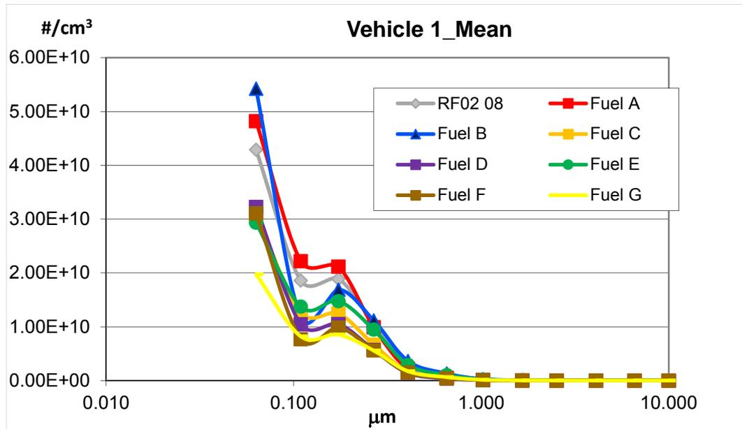
Analysis of the summary histogram plot, **Figure 20** shows the number of particulates is higher with particulates of low diameter, 0.063 µm, 0.109 µm, 0.173 µm, 0.267 µm, decreasing as the diameters increase until the particulate disappears at a size of over 1 µm. As reported above, the single bars represent the arithmetic mean of NEDC test repetitions run for each fuel and the error bars included are the standard deviations calculated for the same set of values.
