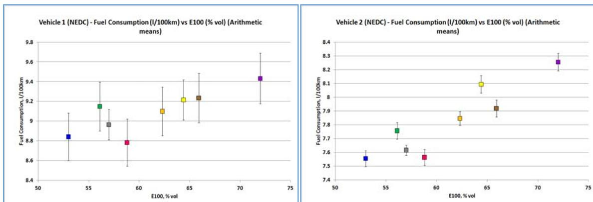
The increase in fuel consumption for two fuels with and without ethanol at 10% and with matched RON is shown in **Figure 24**. There was a significant increase in fuel consumption for Vehicle 2 but not Vehicle 1.
