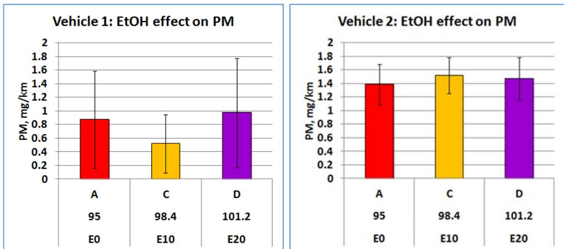
For both vehicles there is no significant difference between the fuels at these low levels. Even with matching RON as shown in **Figure 8** when comparing fuels A and E there was no significant difference. It should be noted that the lack of benefit could be related to insufficient sensitivity of the gravimetric PM measurement method at these low PM levels.
