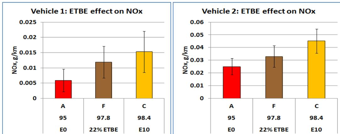
When 98 RON fuel was compared with a 95 RON without oxygenates for Vehicle 2 there was a significant increase in NOx (**Figure 32**).
