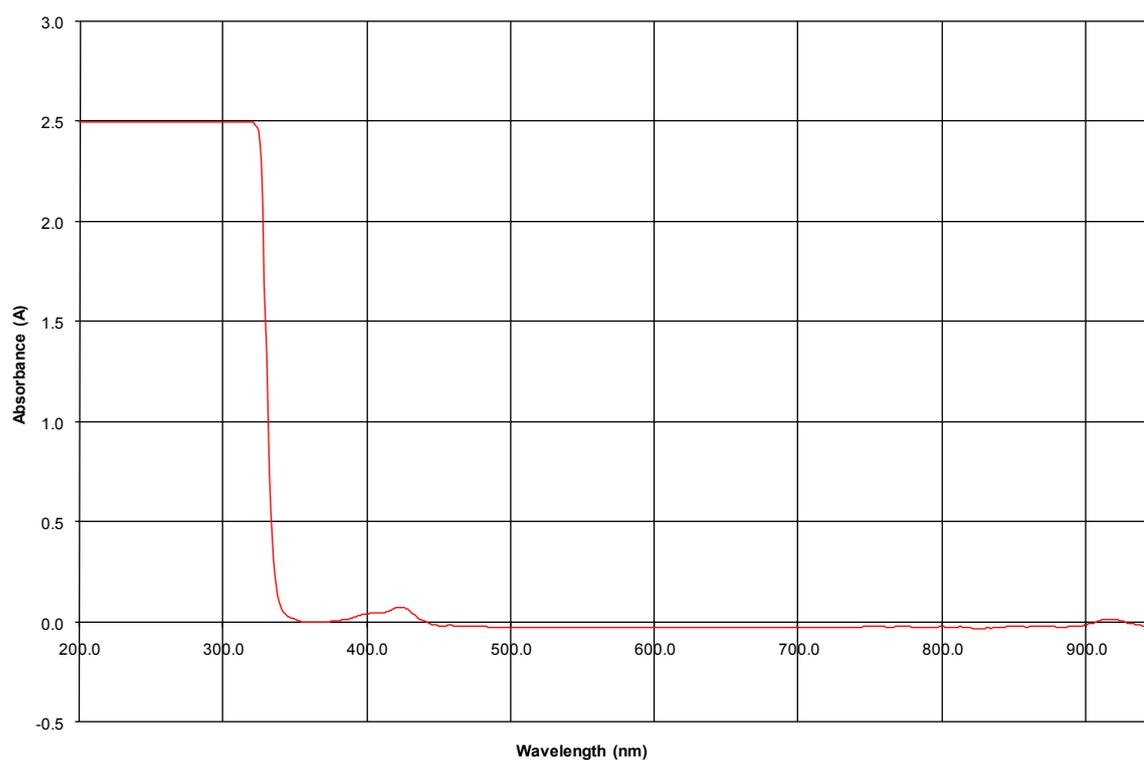
The UV/Visible spectrum shows that the kerosine sample contains aromatic components.
