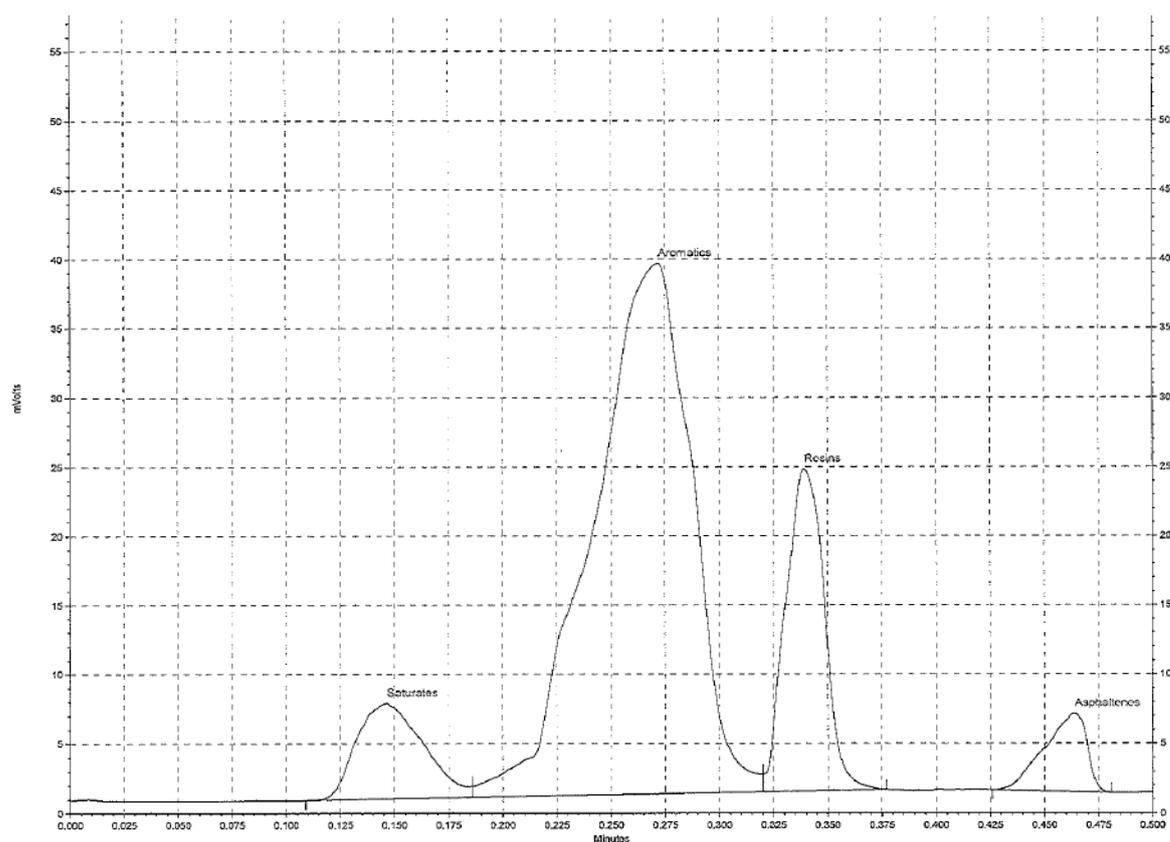
The TLC-FID chromatogram has been annotated to show the peaks corresponding to the saturates, aromatics, resins and asphaltenes present. Normalisation of these peaks showed that the sample contains 10.6% (m/m) saturates, 65.4% (m/m) aromatics, 11.9% (m/m) resins and 12.1% (m/m) asphaltenes.
