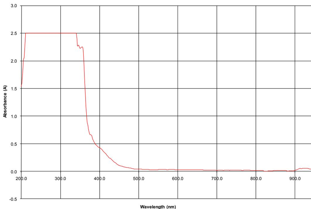
The UV/Visible spectrum shows that the sample contains aromatic components.
