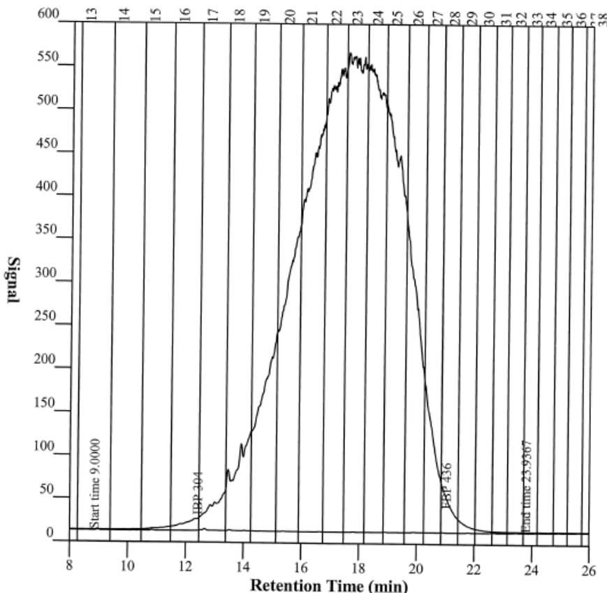
SIMDIS-GC analysis showed that the sample contains hydrocarbons covering the C<sub>15</sub> to C<sub>31</sub> range corresponding with initial and final boiling points of 304°C and 436°C respectively. The boiling point distribution plot and table showing the boiling point for each 5% mass fraction of the sample are shown below.
