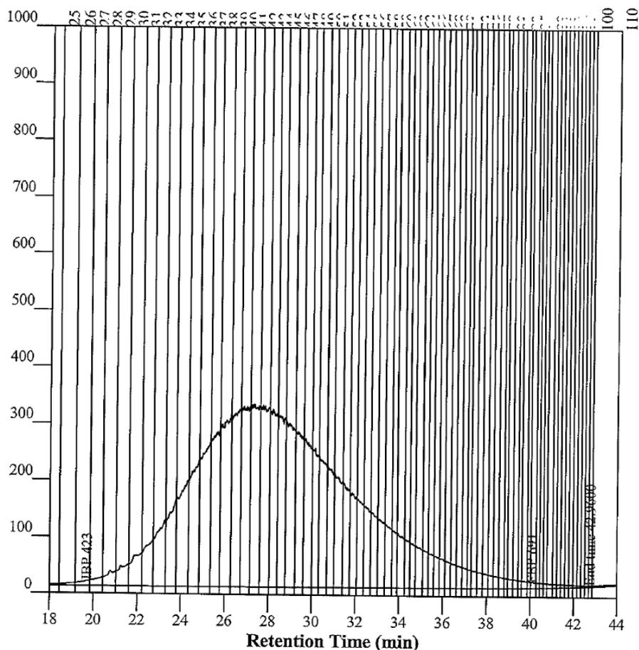
SIMDIS-GC analysis showed that the sample contains hydrocarbons covering the C<sub>25</sub> to C<sub>95</sub> range corresponding with initial and final boiling points of 423°C and 691°C respectively. The boiling point distribution plot and boiling point distribution table for the sample are shown below.
