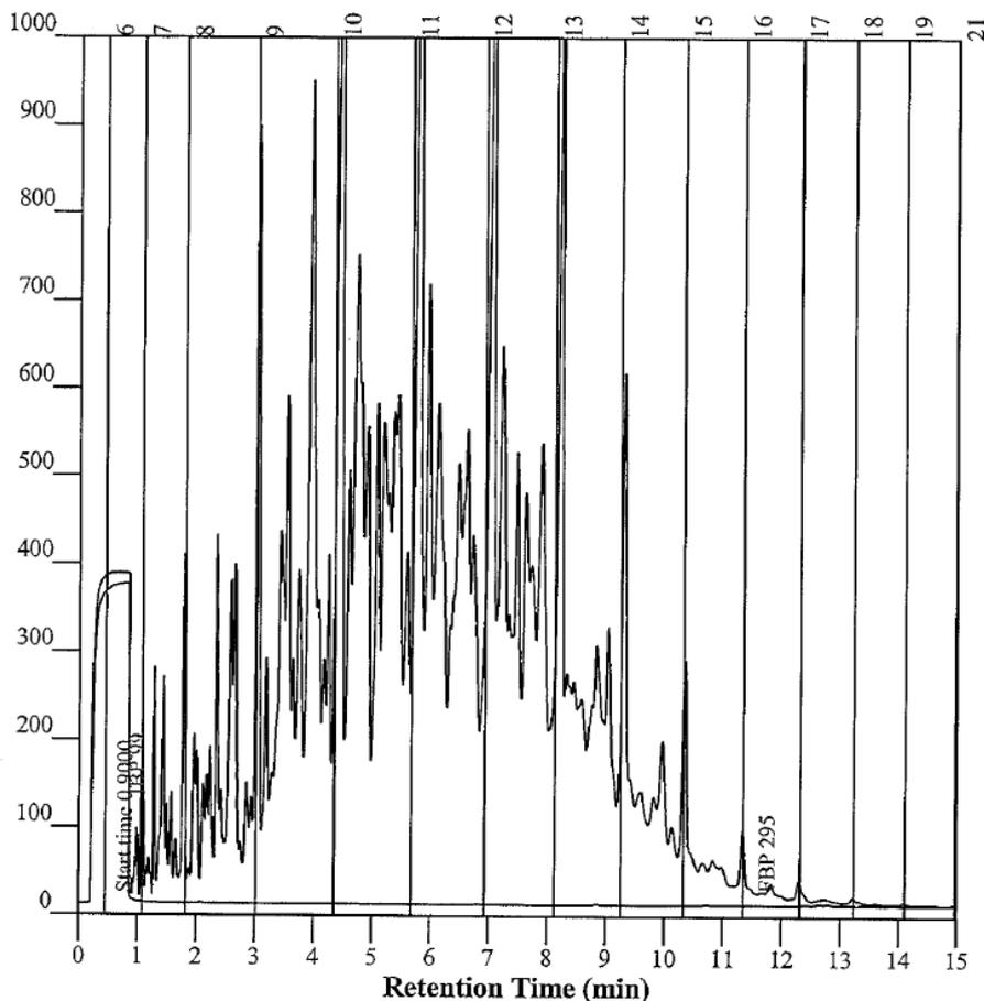
SIMDIS GC analysis shows that the kerosine sample contains components distributed over the C<sub>7-18</sub> carbon number and 99-295°C boiling ranges.
