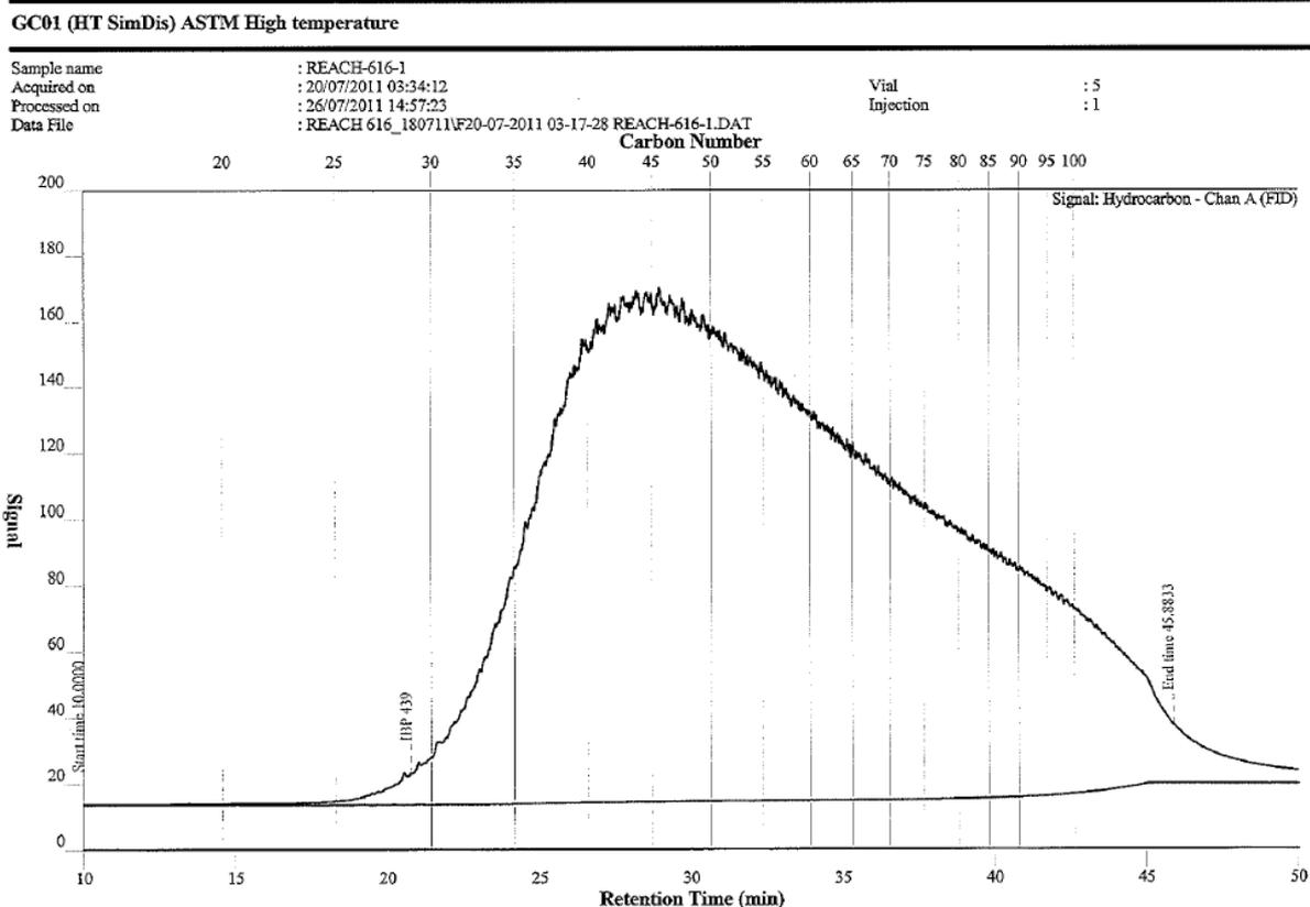
SIMDIS-GC analysis showed that the sample contains hydrocarbons covering the C<sub>25</sub> to >C<sub>100</sub> range corresponding with initial and final boiling points of 439°C and >750°C respectively. The boiling point distribution table for the sample is shown below.
