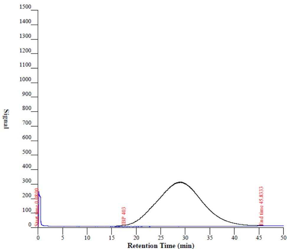
SIMDIS-GC analysis showed that the sample contains hydrocarbons covering the 403°C to >750°C boiling range, although 98% of the sample had a boiling range of 403°C to 702°C. The boiling point distribution table for the sample is shown below.
