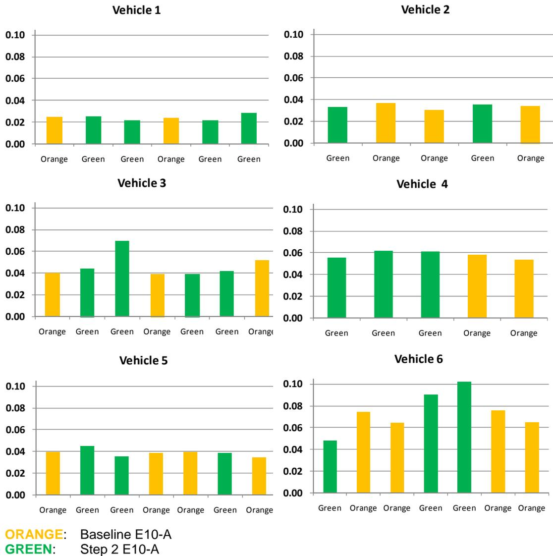
**Figure A2-3** CO emissions (in g/km) over the NEDC at +23°C
