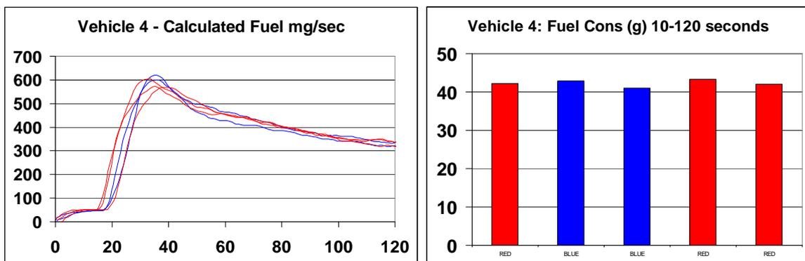
Throttle positions and spark advance were measured for all vehicles except for Vehicle 5 and showed no measureable differences between tests. Under these conditions, the amount of air drawn through the engine should be identical for the two test fuels. Direct measurements of mass air flow on Vehicles 1 and 2 (the only
