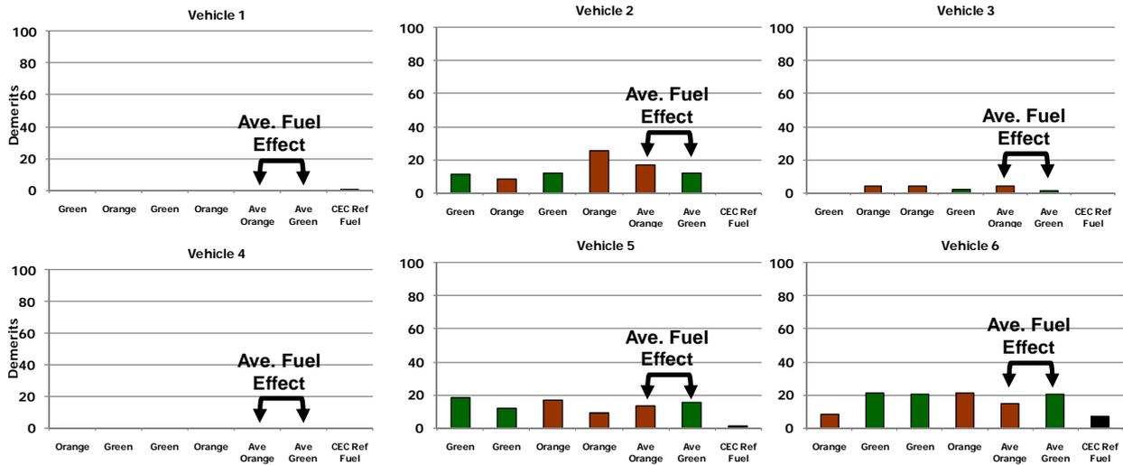
Figure 3.6.2 adds idle instability demerits. Still, three of the vehicles showed low demerits, below 24, while Vehicle 2 had one test on the Baseline E10-A (ORANGE) fuel with 33 demerits. Vehicle 5 showed very high levels of idle instability demerits, due primarily to “flaring” of the engine speed when returning to idle. Five of the vehicles had substantially lower average demerits on the Step 2 E10-E (GREEN) fuel while one (Vehicle 3) had very low and similar demerits on both fuels.
