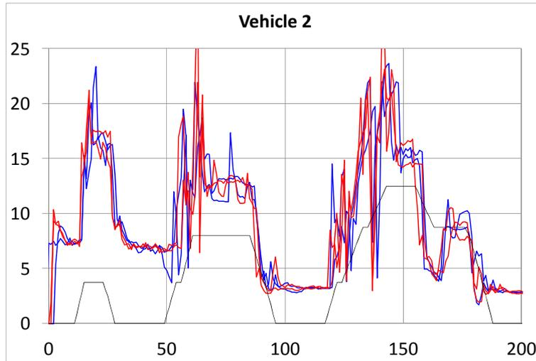
**Figure 3.4.12** Throttle position signal from the EMS over ECE-1 following cold engine starting at -7°C, for Vehicle 2. The x-axis is the time in seconds after cold engine starting.
