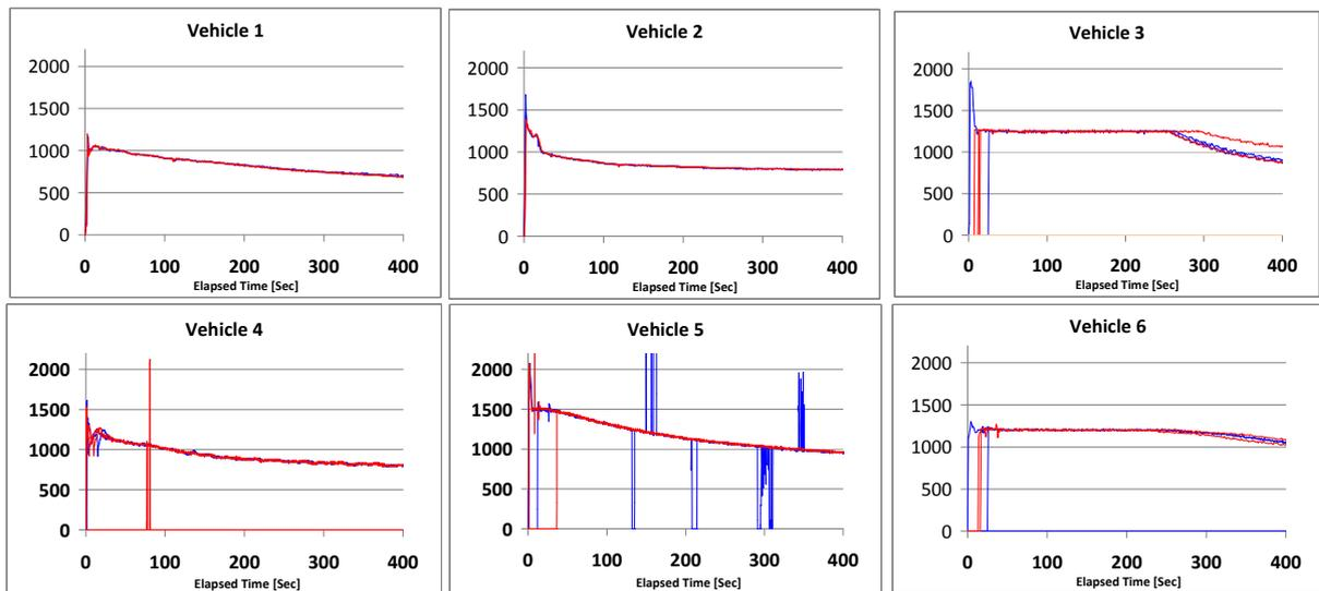
Results are shown for the first 400s of the test. All the vehicles started easily (<1.6s) on both fuels and followed the same profile of high initial idle speed which decreased steadily as the engine warmed up. Engine speed profiles were consistent between tests (the occasional spikes in the traces represent temporary noise in the measuring system). Where there was some evidence of test to test variation (Vehicles 3 and 6), it appeared randomly and there was no evidence of a fuel effect.
