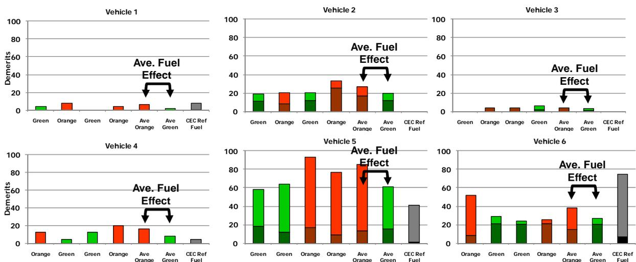
**Figure 3.6.3** HWD Demerit ratings at +40°C for (1) stumbles and surges, (2) idle instability, and (3) longer acceleration times. The CEC Reference fuel was not tested on Vehicles 2 and 3.
