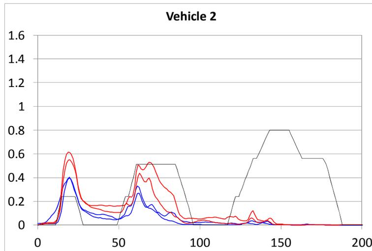
**Figure 3.4.8** Instantaneous FC [in g/s] over ECE-1 following cold engine starting at  $-7^{\circ}\text{C}$ , for Vehicle 2. The x-axis is the time in seconds after cold engine starting.
