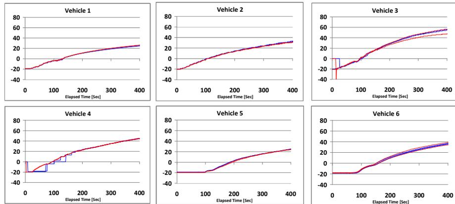
Coolant thermocouples were located in the top hose of the test vehicles (i.e. the ‘cold’ side of the thermostat). In spite of this, recorded temperatures started to rise very shortly after engine start and had reached 25-50°C after 400s. Temperatures generally followed consistent profiles for each test. Vehicles 3 and 6 again showed a small degree of test-to-test variability but this was not related to the fuel type.
