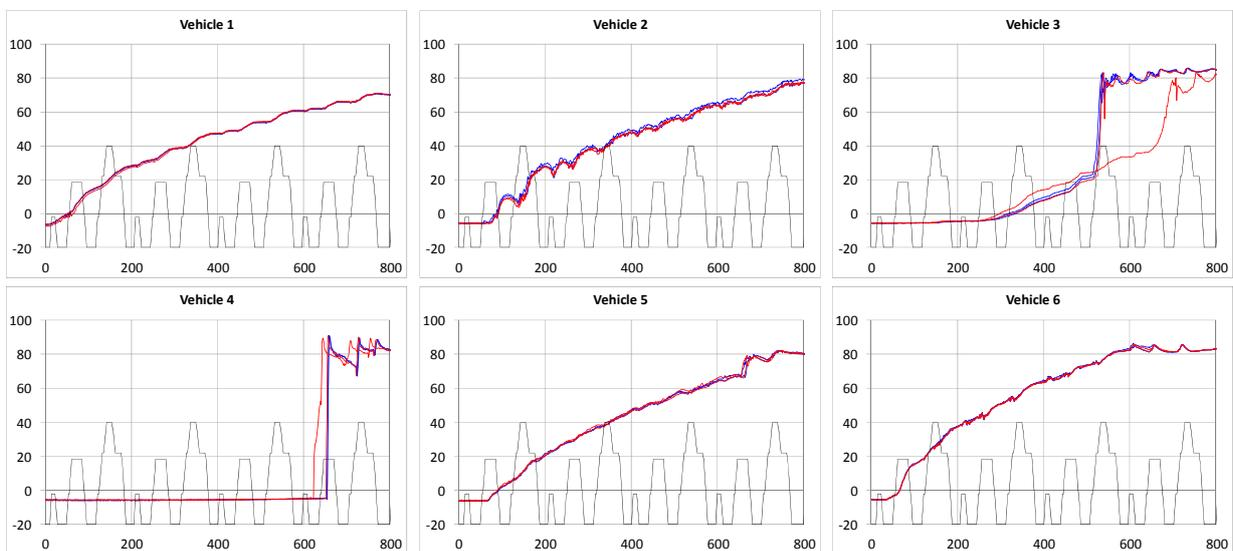
The measured oil temperature shows more comparable responses between the vehicles, and is generally slower than the coolant temperature rise, apart from Vehicle 2 where the two temperatures follow very similar profiles. The temperatures at the end of the ECE phases ranked the vehicles in the following order: Vehicles 3, 2, 4, 6, 5 and 1. This ranking does not generally correlate with any simple vehicle metric such as size or inertia class. The temperature responses were not fuel dependent.
