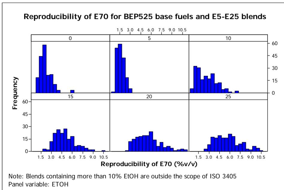
It can be seen that the reproducibility in general gets markedly worse as the ethanol concentration increases and the distillation curves get flatter and less precisely defined at the 70°C point. Interestingly, however, the slopes at 70°C are slightly steeper for E5 blends than they are for BOBs (see, for example, **Figure 1.1** in **Section 1.1.1**), hence the slightly better precision for E5 blends.
