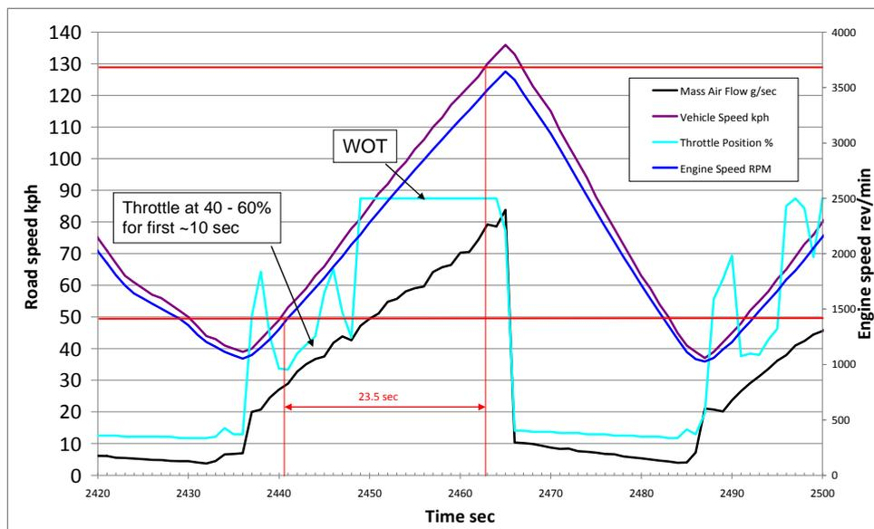
**Figure A6-5** Full throttle acceleration in 5<sup>th</sup> Gear for Vehicle 1 on Step 2 E10-A (GREEN) fuel
