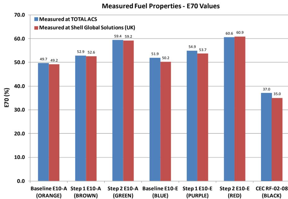
**Figure A7-4** Comparison of E70 results on different samples of the same fuel blends, measured at Total ACS (in Givors, France) and Shell Global Solutions (UK) (in Thornton, UK)
