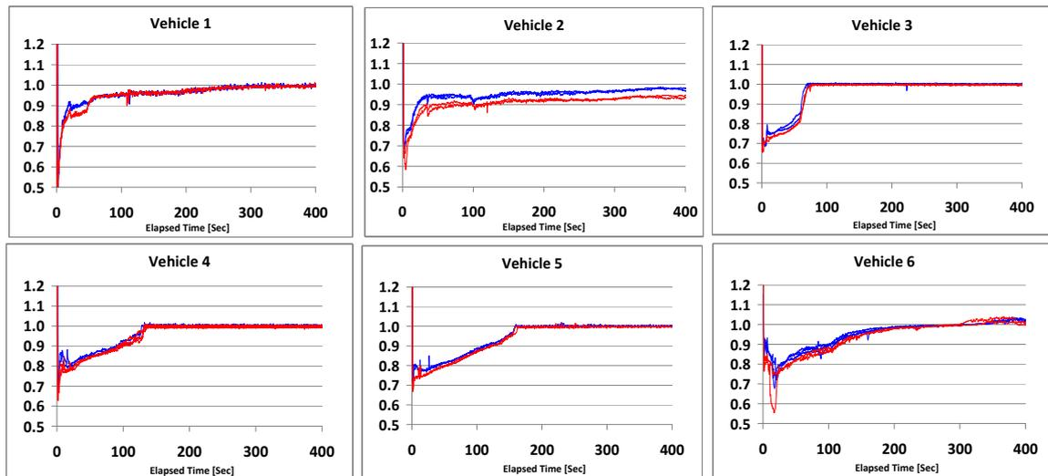
A clear transition from open-loop operation to lambda control was seen for Vehicles 3, 4, and 5 while the other vehicles approached lambda=1 in a more ambiguous way. Vehicle 2 appeared to reach lambda control around 50s but remained slightly rich of lambda=1 throughout the 1200s test. Vehicle 6 appeared to trend lean after a period of lambda=1 operation. The fuel did not affect the time taken to reach lambda control.
