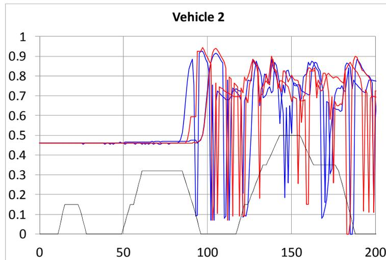
**Figure 3.4.11** Mass air flow signal from the EMS over ECE-1 following cold engine starting at -7°C, for Vehicle 2. The x-axis is the time in seconds after cold engine starting.
