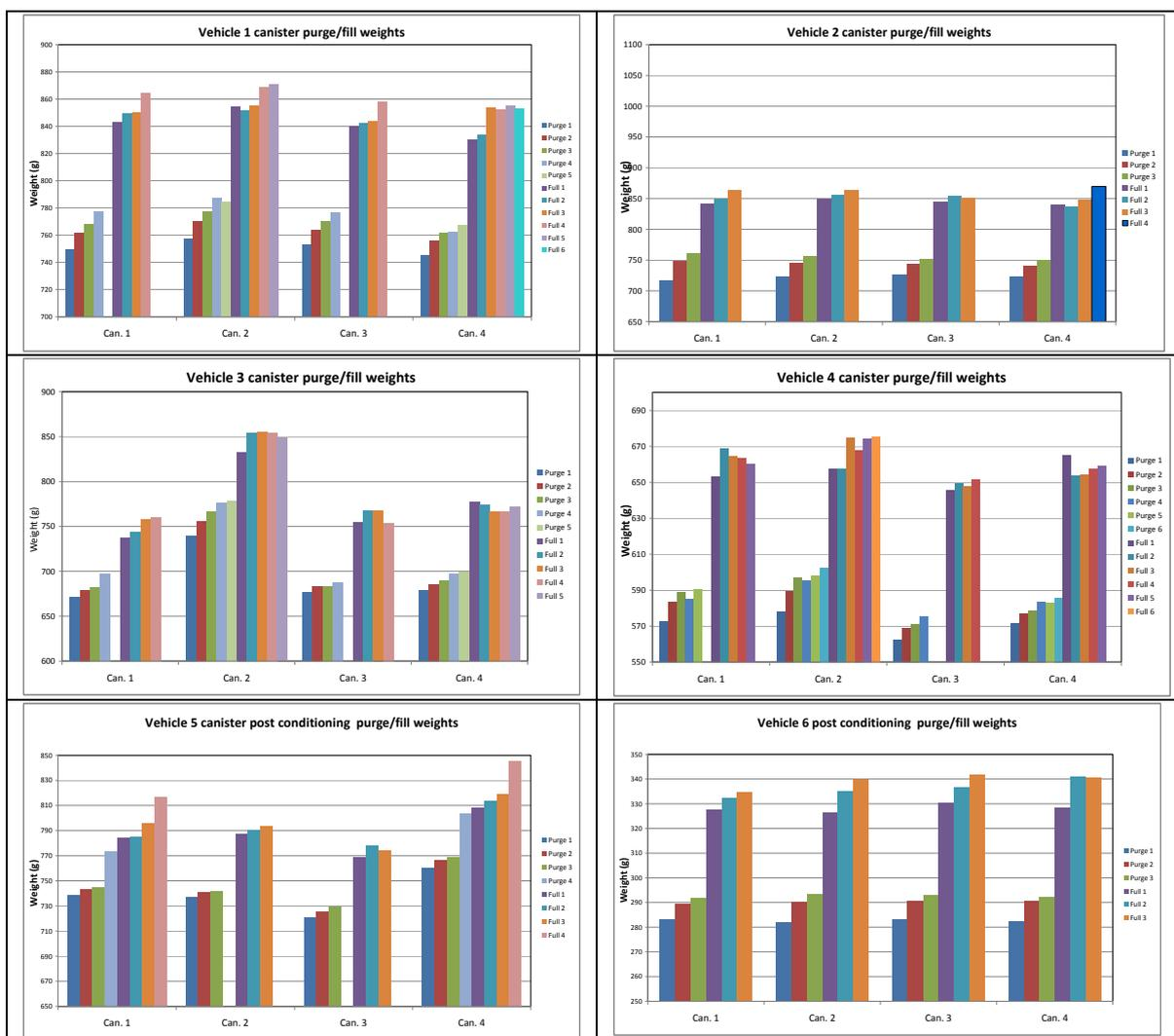
**Figure A5-3** Canister working capacity
