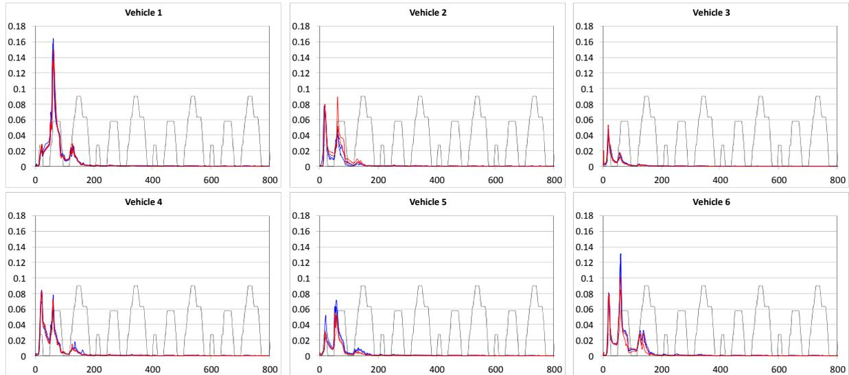
The CO emissions are shown in **Figure A4-8**. Similar to THC, the vehicles tend to show two or three peaks in CO emissions corresponding with the first three acceleration phases of the ECE. After the first 200s, the CO emissions are generally low, although a couple of vehicles show some small spikes during transients, suggesting over-rich combustion mixture. Vehicle 2 shows higher CO emission rates from the more volatile RED fuel.
