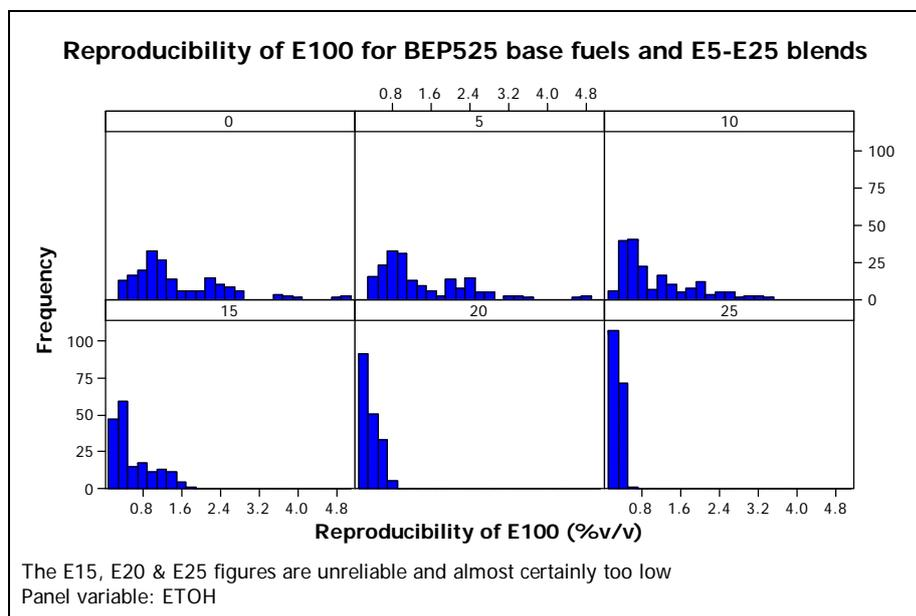
The reproducibility 'R' is found to be very low for E20 and E25 blends and to a lesser extent for E15 blends. However, Annex C of ISO 3405 states that the method of calculation of the repeatability and reproducibility of Exxx values is not reliable when the slope dT/dV is high. From the plots in Appendix 8 of [10], it can be seen that the distillation curves are very steep at T=100°C at higher ethanol concentrations. In fact, Annex C of ISO 3405 quotes a general reproducibility figure
