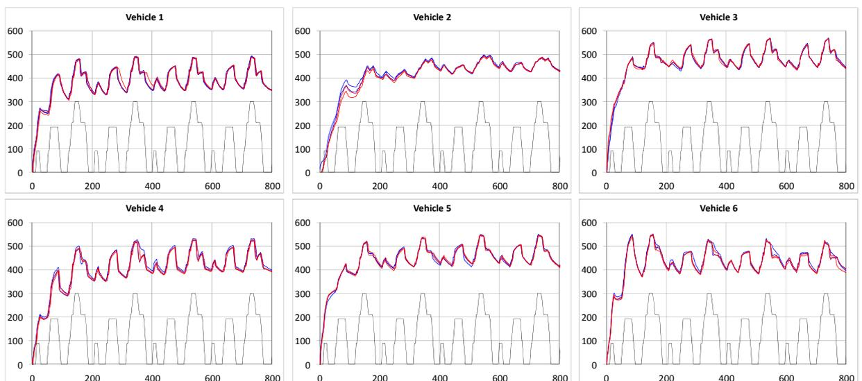
**Figure A4-5** Post-catalyst temperature during ECE following cold engine starting at -7°C (except for Vehicle 1 – see text)
