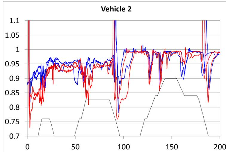
**Figure 3.4.10** Manufacturer-installed lambda sensor signal over ECE-1 following cold engine starting at -7°C, for Vehicle 2. The x-axis is the time in seconds after cold engine starting.
