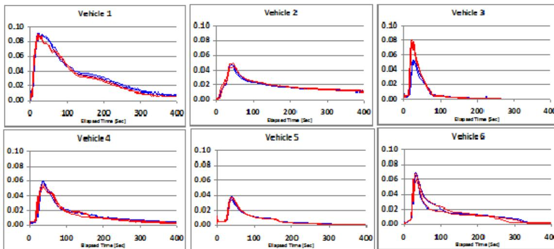
For the CO emissions, peak values ranged from 7% to 11% and were all within the range of the exhaust analyser. Results in g/second are shown in **Figure A3-5**.
