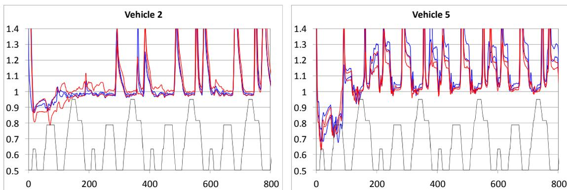
**Figure A4-13** Exhaust gas  $\text{CO}_2$  concentration [ppm] during ECE following cold engine starting at  $-7^\circ\text{C}$
