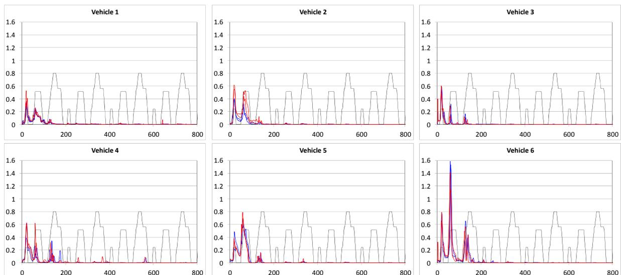
The NOx emissions are shown in **Figure A4-9**. The results are more vehicle dependent than the THC and CO, so no general trends are evident. Several of the vehicles show the highest NOx emissions within the first 100 seconds, beyond which the NOx emissions are negligible. However, Vehicle 3 shows spikes of NOx emissions throughout the test and Vehicle 5 shows extremely low levels of
