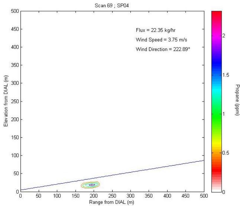
**Figure 5b** Visualisation of emission rate for Scan 69 representing SP04/LOS1
