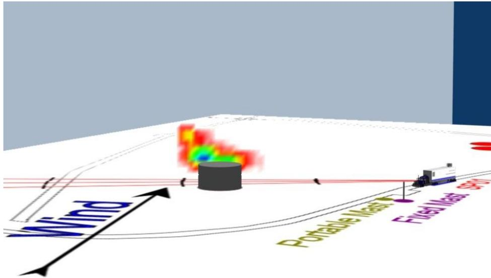
**Figure 5a** Observed propane concentration for Scan 69 representing SP04/LOS1
