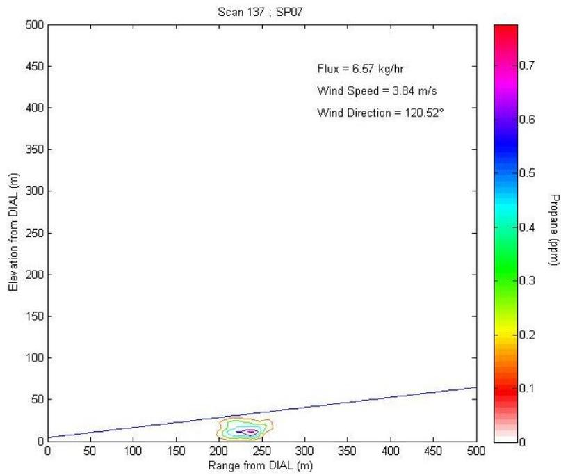
**Figure 6b** Visualisation of emission rate for Scan 137 representing SP07/LOS3
