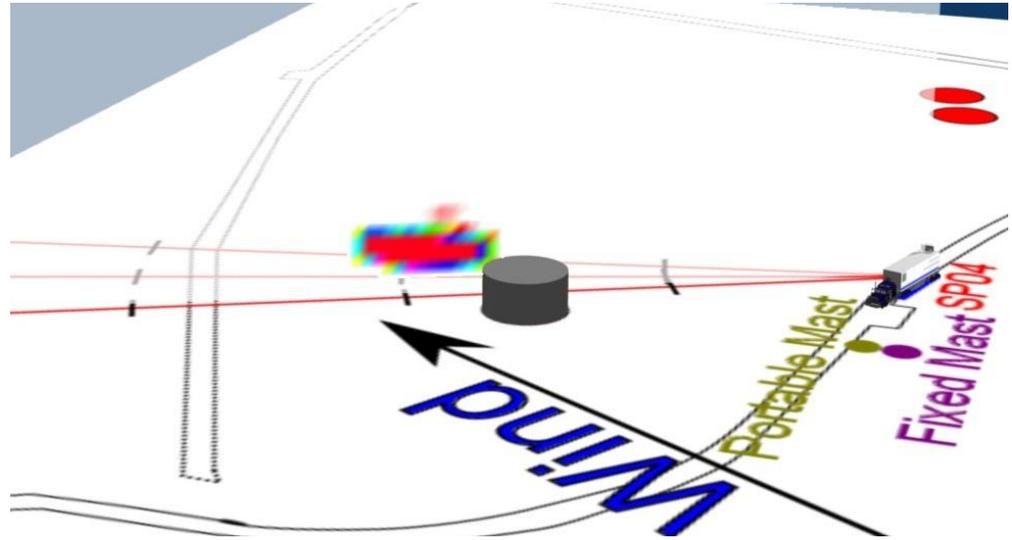
**Figure 6a** Observed propane concentration for Scan 137 representing SP07/LOS3
