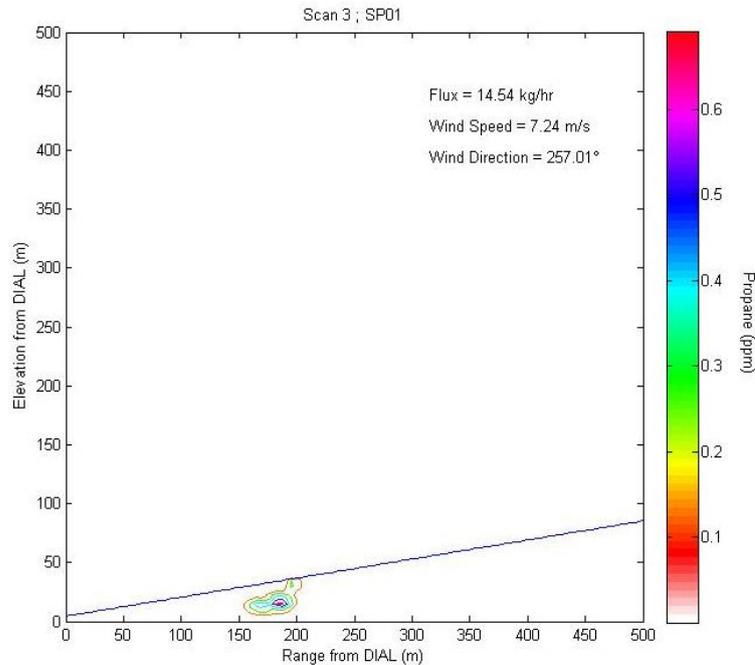
**Figure 4b** Visualisation of emission rate for Scan 3 representing SP01/LOS1
