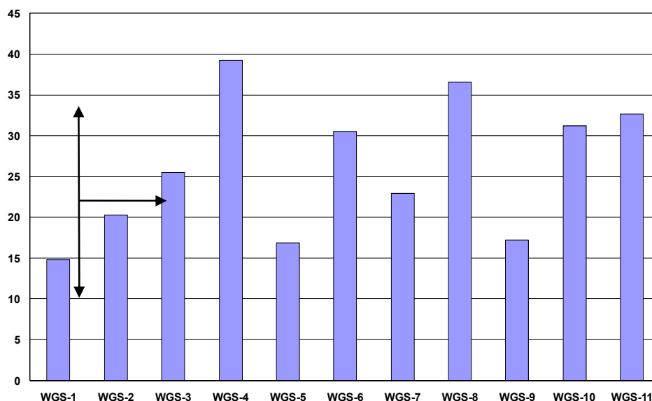
Figure 8 Distribution of Wet Gas Scrubbing Costs within the Cost Survey data. All costs scaled to a unit size of 2 Mt of fresh feed per year. The mid value (26 M€) and range (16-36 M€) are indicated
