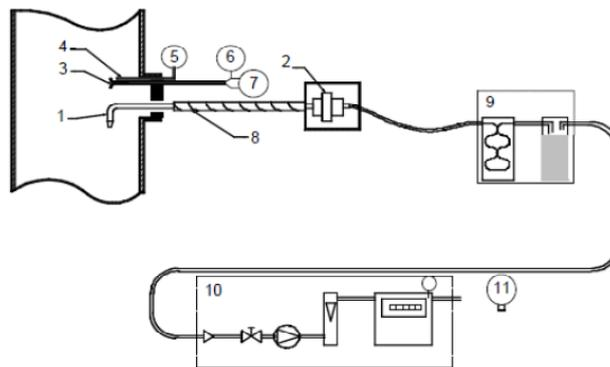
**Figure 3: Example of a manual dust sampling as illustrated in the EN 13284-1. The sampling line is heated and the filter is located outside the stack (2 on the scheme).**
