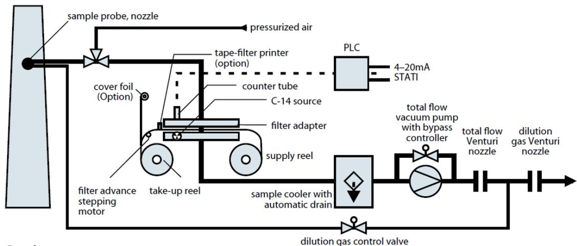
Figure 8 : Operating principle of a Beta gauge monitor with dilution of the sample (Verewa Beta gauge monitor F-904-20, Durag catalogue).
