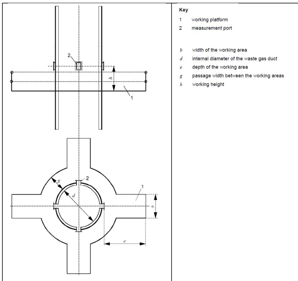
**Figure 10: Example of a working platform and the position of measurement ports in a vertical round waste gas duct (source: EN 15267, figure A.7).**
