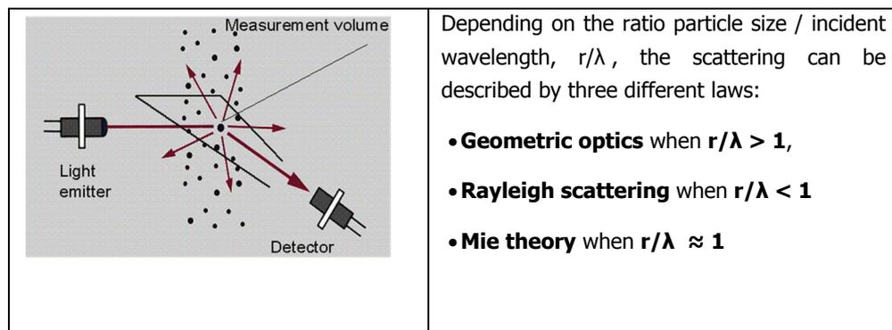
**Figure 5 : Illustration of the light scattering by a particle in all the directions.**
