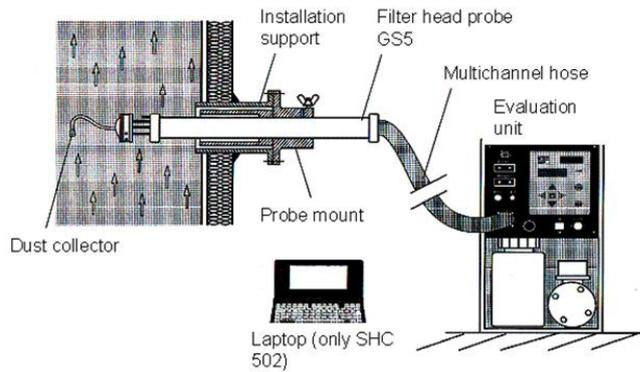
**Figure 2: Example of manual dust sampling with a GRAVIMAT (SICK company). The filter is located in the head of the sampling probe inside the stack.**
