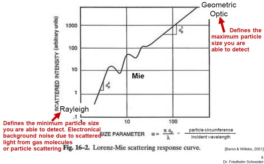
**Figure 6 Physical background- scattering intensity vs. particle size/wavelength (Grimm presentation).**
