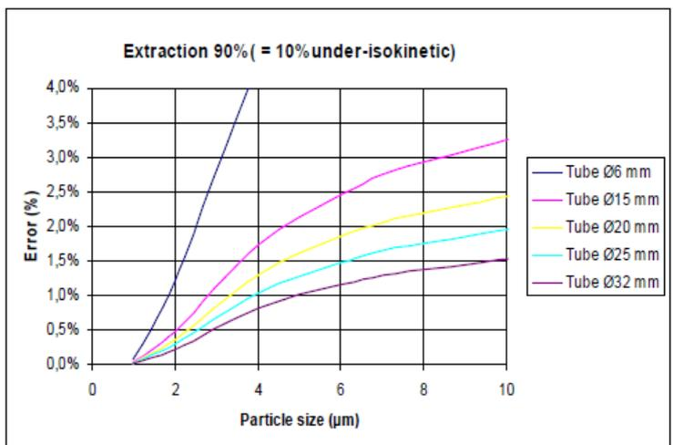
b. Illustration of under-isokinetic sampling and its effects on final result
