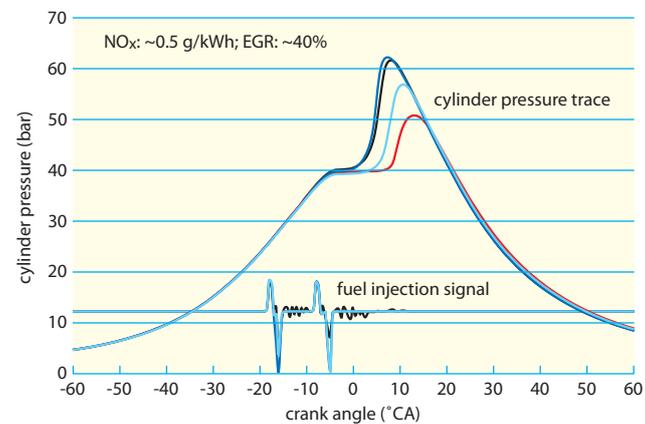
*Lowering the fuel's cetane number delays the peak combustion pressure.*
