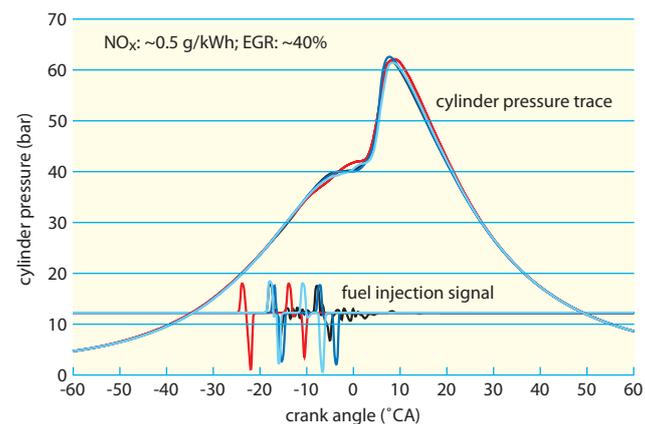
*Adjusting the injection timing for each fuel optimises the combustion pressure.*
