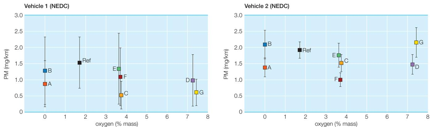
Figure 5 PN emissions versus oxygen content (geometric means)
