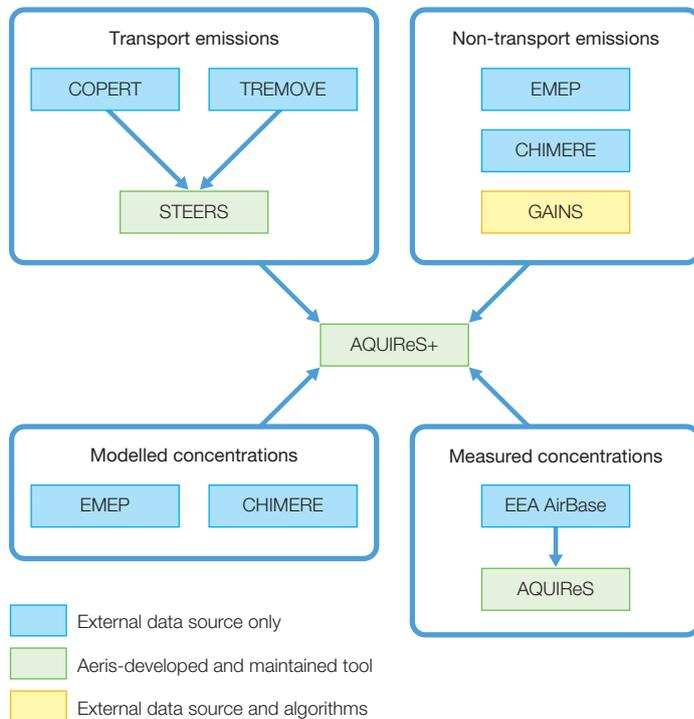
The robustness of the modelling approach was verified by hind-casting and comparing the predicted concentration levels with historical measurement data from the EEA AirBase database. The tools used in this study are shown in Figure 2.
