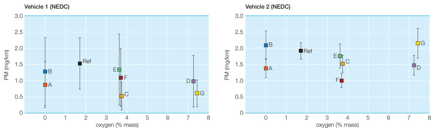
Figure 5 PN emissions versus oxygen content (geometric means)
