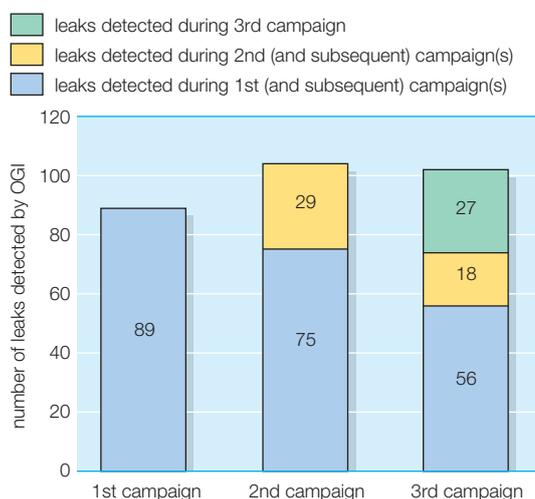
In the same way, successive sniffing campaigns also point out differences in the leak screening values. But as OGI surveys are faster, it is possible to increase campaign frequency at similar cost and improve leak detection effectiveness.
