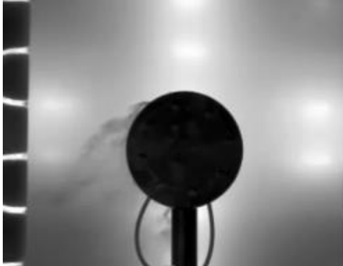
Large leak area (diffused leak)
