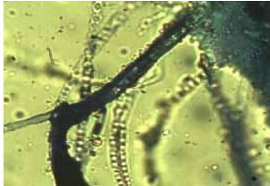
fungi hyphae in the diesel fuel phase (yellow), extend into water phase (dark), ca. 800x
