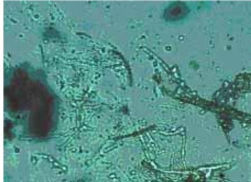
fungi hyphae and micro water droplets in the fuel phase, ca. 800x
