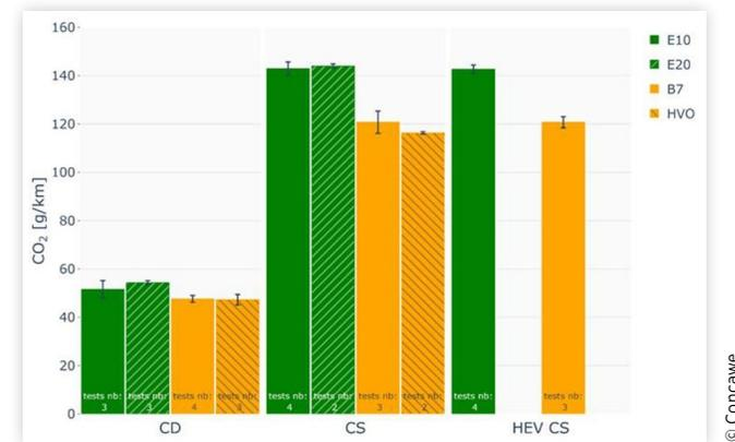
**FIGURE 16** Comparison of corrected tailpipe CO<sub>2</sub> emissions [g/km] measured on RDE cycles on chassis dyno for each fuel and mode.
