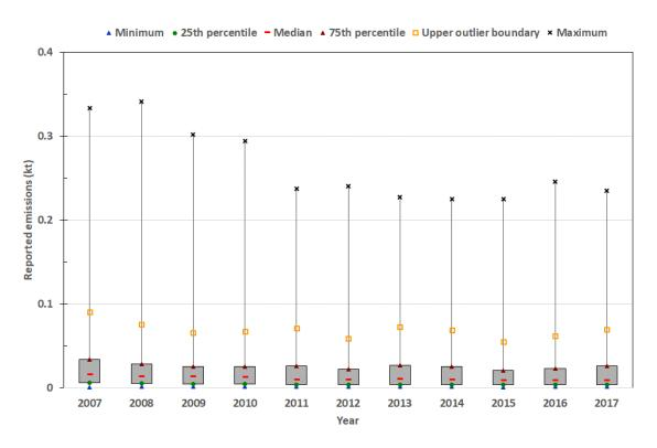
Figure 29 Statistical analysis of benzene air emissions for European refineries: 5<sup>th</sup> and 95<sup>th</sup> percentiles
