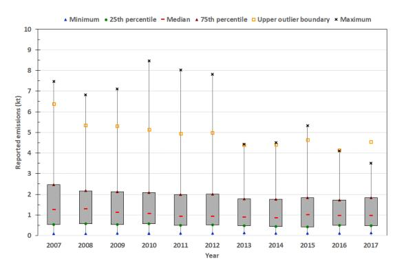
Figure 13 Statistical analysis of nitrogen oxides air emissions for European refineries: 5th and 95th percentiles
