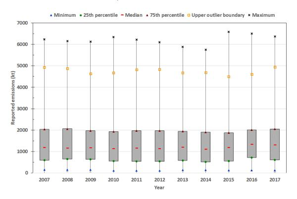
Figure 37 Statistical analysis of  $CO_2$  air emissions for European refineries:  $5^{th}$  and  $95^{th}$  percentiles
