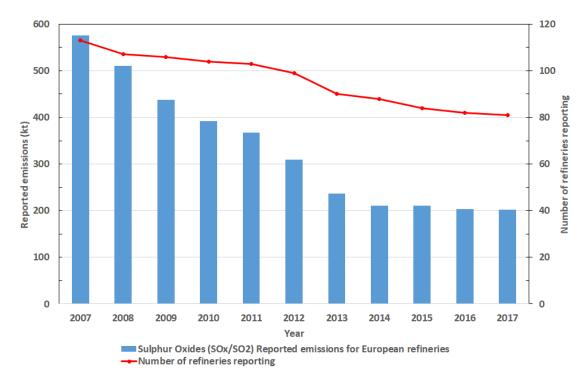
**Figure 3** Trends of oxides of sulphur air emissions reported for European refineries during 2007-2017, expressed as per unit of crude processed
