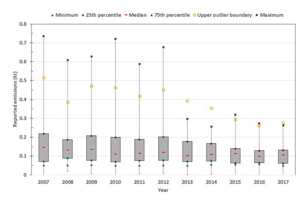
Figure 45 Statistical analysis of  $PM_{10}$  air emissions for European refineries:  $5^{th}$  and  $95^{th}$  percentiles
