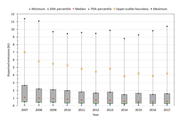
Figure 21 Statistical analysis of NMVOCs air emissions for European refineries: 5th and 95th percentiles
