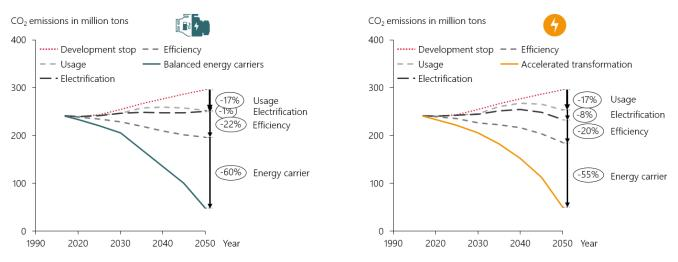
Figure 5: Comparison of CO<sub>2</sub> emission reduction in the Balanced Energy Carriers (left) and Accelerated Electrification (right) scenarios in a well-to-wheel balance.
