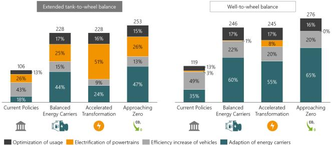
CO<sub>2</sub> emission reduction in million tons and breakdown by measures
