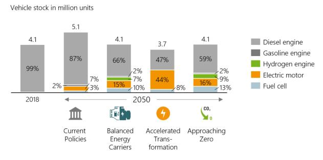
Figure 4: Heavy-duty vehicle stock in million units, shown by main energy conversion system in 2018 and 2050 in the four scenarios.
